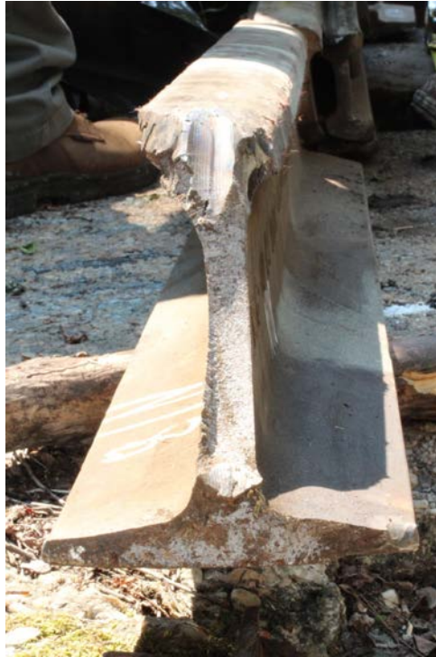
Figure No. 6. A view of a severe wheel flange strike mark on piece No. “N 18”.
