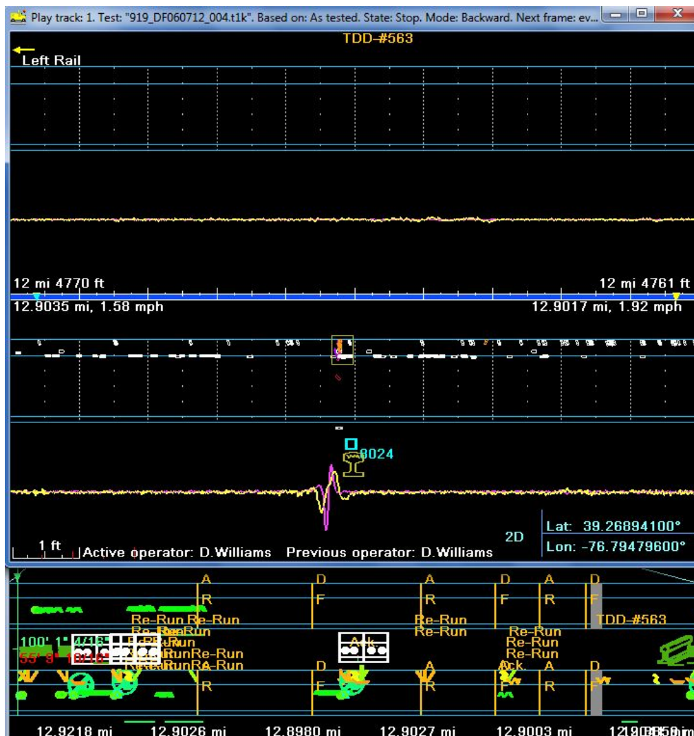
Figure No. 12. July Test Car Re-runs and defect location.
