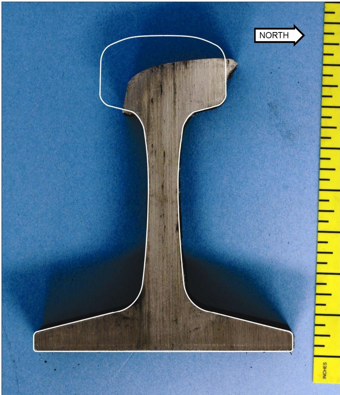
Figure 16. View of the rail cross-section (as-cut surface) near the west end of piece N5. The outline represents the cross-section of a new 136 pound rail.
