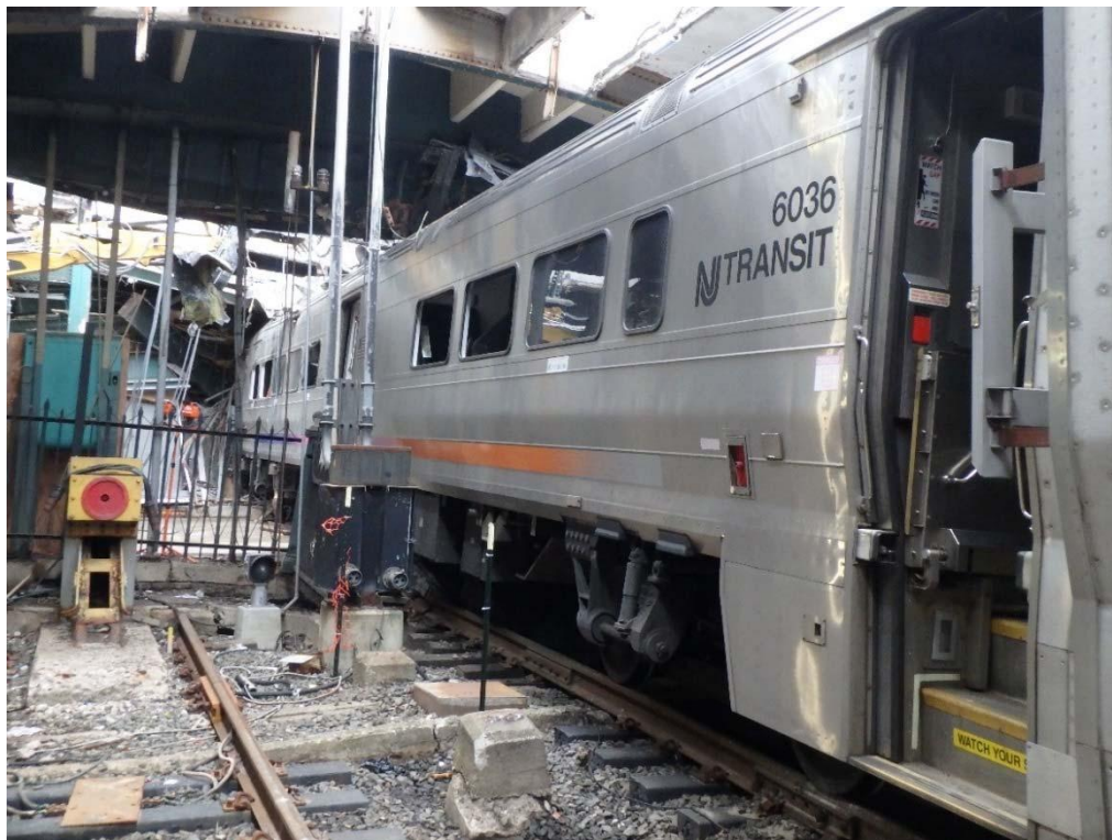
10 Figure 1. Controlling cab car of accident train shown beyond the end of the track and at rest against 11 the station wall. Damage to the station structure also shown, with a portion of the canopy resting on 12 the accident train (Photo NTSB)
