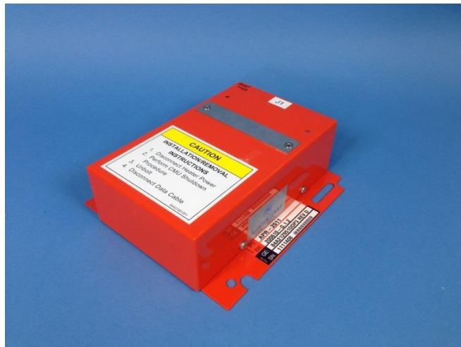
Figure 1. GE LocoCAM Hard Drive from BNSF Locomotive 7750.
