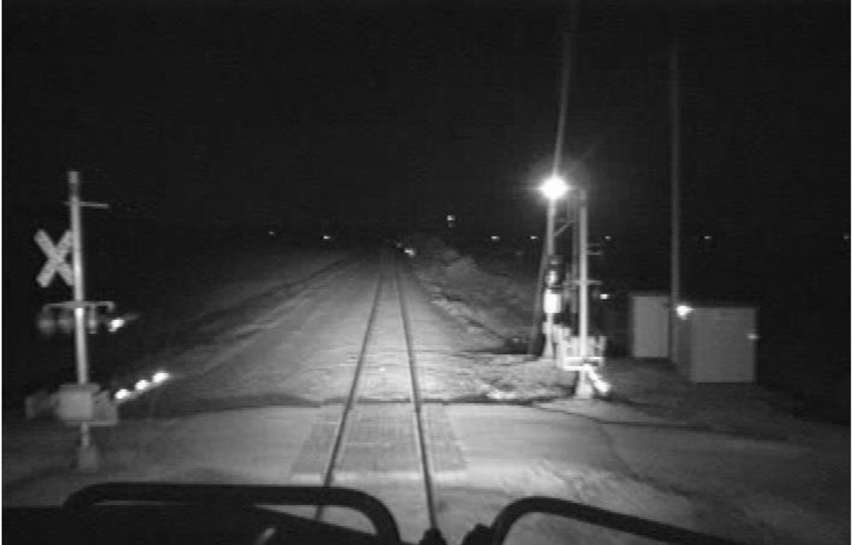
Figure 13. A horn is heard as the locomotive passes a private grade crossing at a flashing yellow Intermediate Signal (Milepost 127.7).
