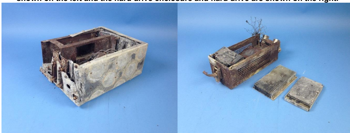
Figure 21. The arrival state of UP locomotive 7421's image recorder. The recorder chassis is shown on the left and the hard drive enclosure and hard drive are shown on the right.
