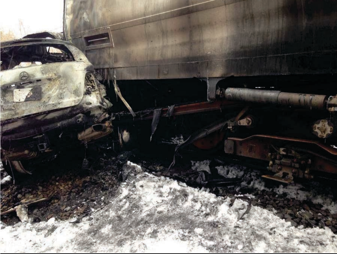
Figure 8-West side view of the third rail passing through the SUV and entering passenger car MN 4333.
