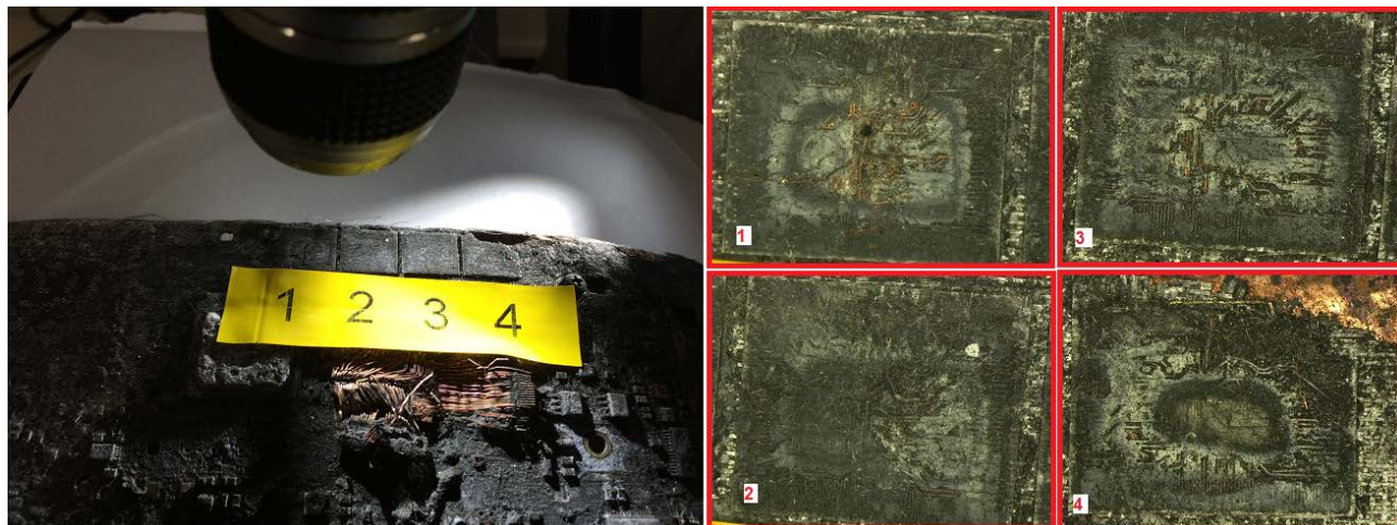
Figure 2. Internal board with NVM chips annotated.
