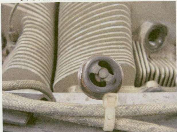
71. SPARK PLUG AFTER RIGHT FUEL SYSTEM RUN ON LEFT ENGINE
