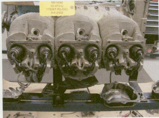
26. LEFT CYLINDER OVERHEADS
