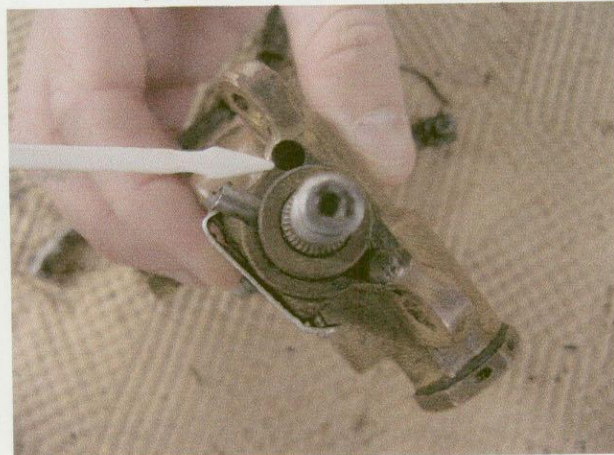
64. MISSING STOP PIN
