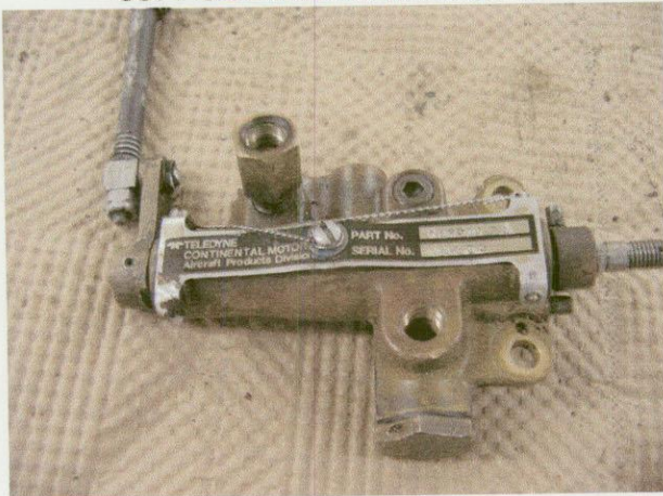
63. FUEL METERING UNIT
