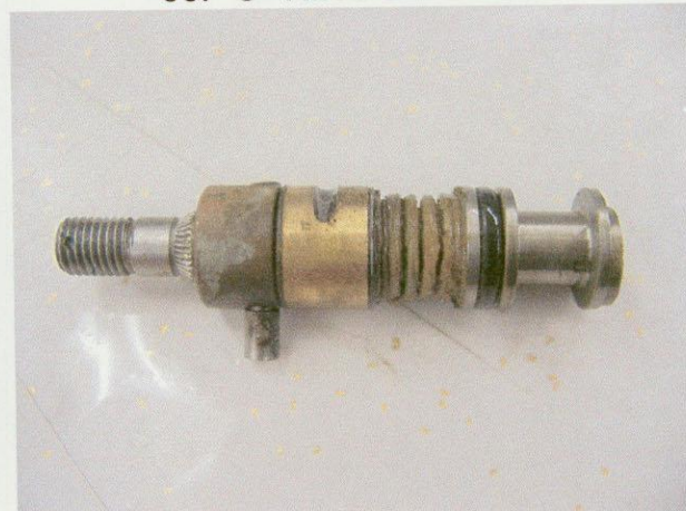
66. "O" RING LEAKING
