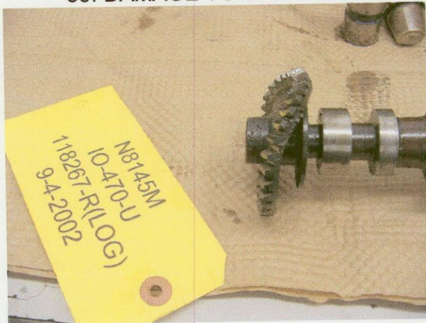
35. DAMAGE TO CAM GEAR
