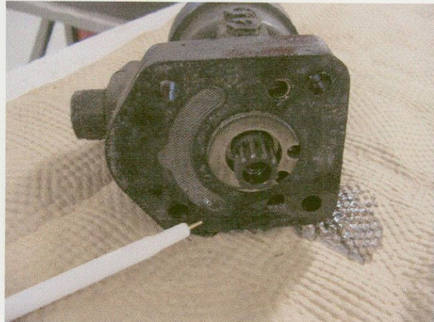
18. DEBRIS FOUND IN SCREEN AT POINTER
