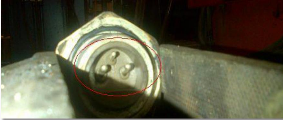
Pins bent upwards
