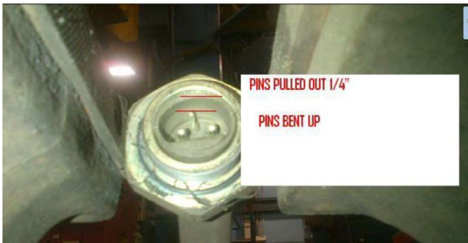
Pins pulled out 1/4" and bent up
