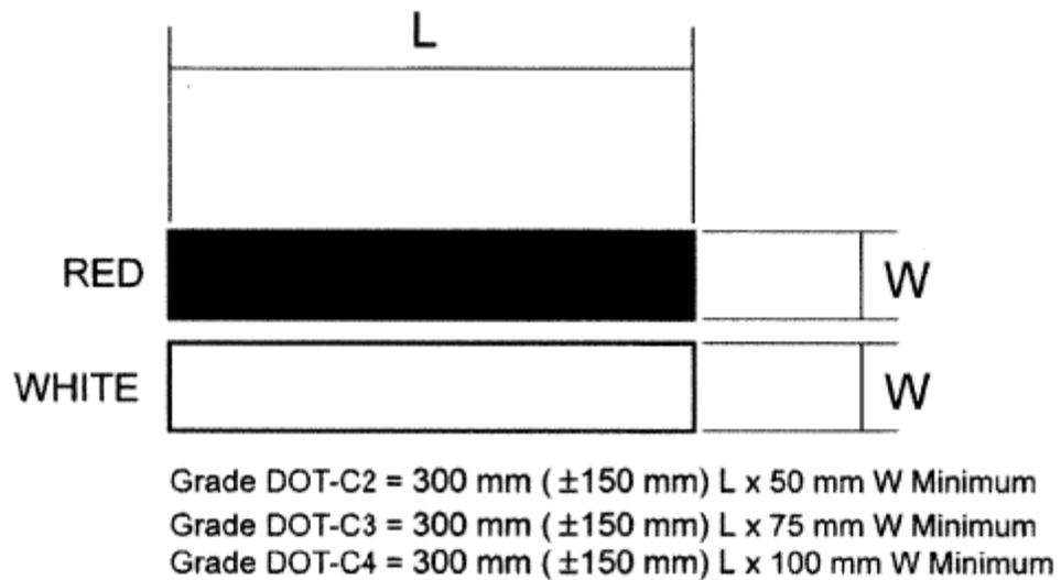
Figure A2-2: Partial copy of FMVSS 108 Figure 12-1 depicting minimum size requirements for retroreflective sheeting panels.
