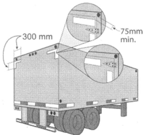
Figure A2-3: Partial copy of FMVSS 108 Figure 11 depicting requirement for placement of retroreflective sheeting panels on van body semitrailers.
