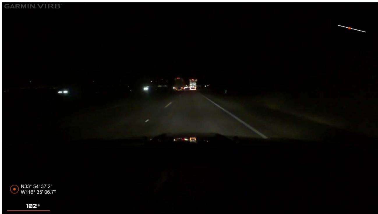
Figure 4: Video image capture depicting the approach to several semitrailers along an unlit portion of the highway. The separation distance is approximately 550-600 feet with low beam headlights in use. Both semitrailers exhibited rearward facing retroreflective sheeting, while the semitrailer occupying the right lane also featured stainless-steel rear door skin. (Video recorded in high definition, 1080p, at 30 frames per second with a 14mm equivalent lens focal length.)
