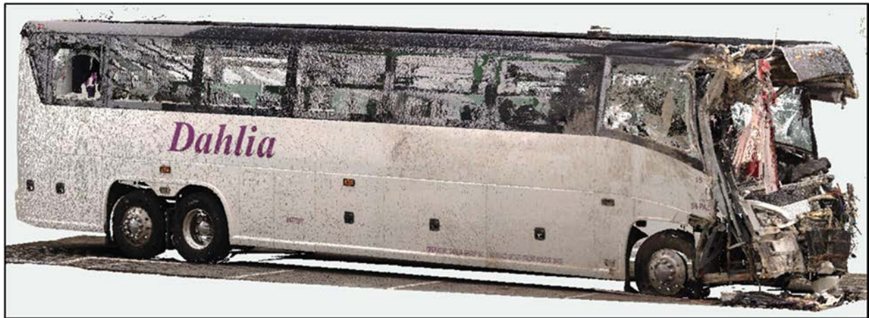
Figure 4: Depiction of linked 3D scans of the involved MCI motorcoach from the passenger side.
