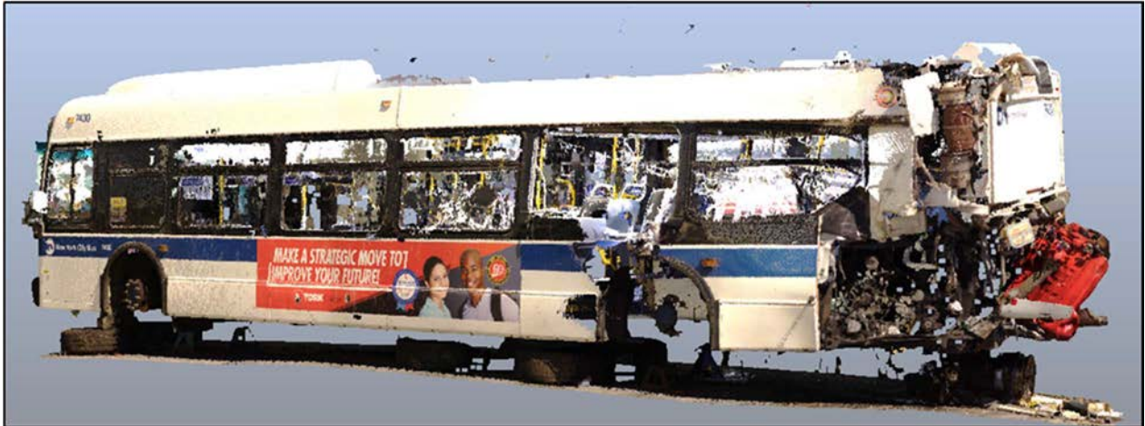
Figure 8: Depiction of linked 3D scans of the MTA New Flyer transit bus involved in the collision.
