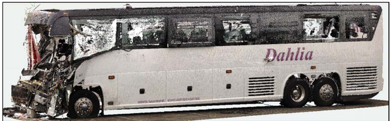
Figure 5: Depiction of linked 3D scans of the involved MCI motorcoach from the driver side.
