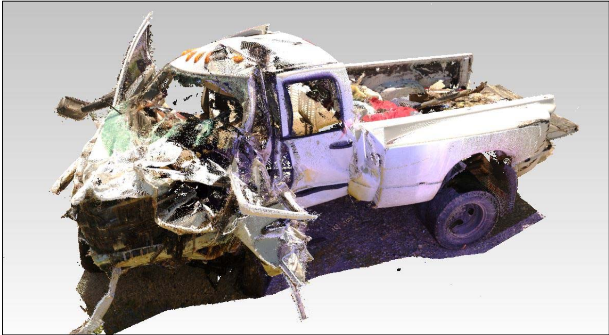
Figure 5: The image depicts linked 3D scans of the Ford bus as viewed looking toward the left front of the vehicle where the impact damage was concentrated.
