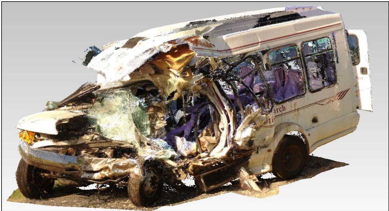
Figure 3: The image depicts linked 3D scans of the Ford bus as viewed looking toward the left front of the vehicle where the impact damage was concentrated.
