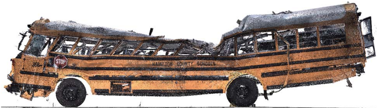
Figure 3: Image of 3D scan point cloud depicting the left (driver's side) of involved bus after removal from the scene. Scan data was provided by CPD.
