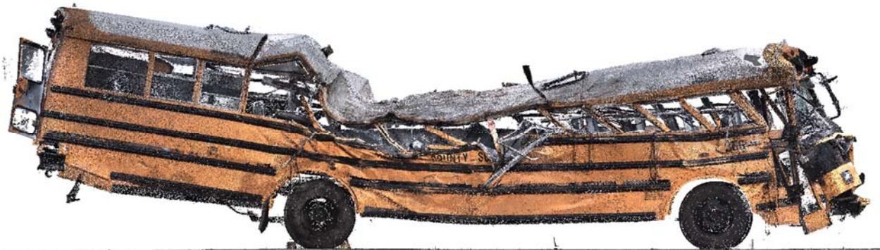
Figure 4: Image of 3D scan point cloud depicting the right (passenger's side) of involved bus after removal from the scene. Scan data was provided by CPD.
