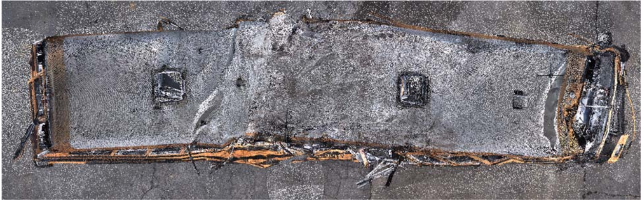
Figure 5: Image of 3D point cloud depicting an overhead view of involved bus following its removal from the scene. Scan data was provided by CPD.
