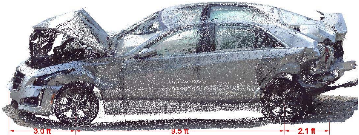
Figure 25: Point cloud image of the Cadillac depicting certain dimensions.
