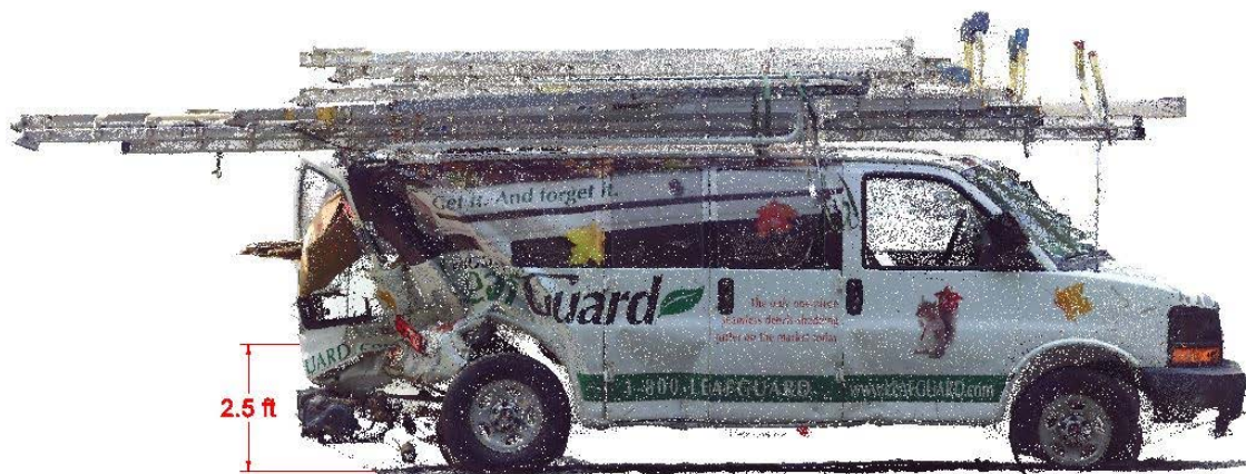
Figure 15: Point cloud image of the GMC van depicting certain dimensions.
