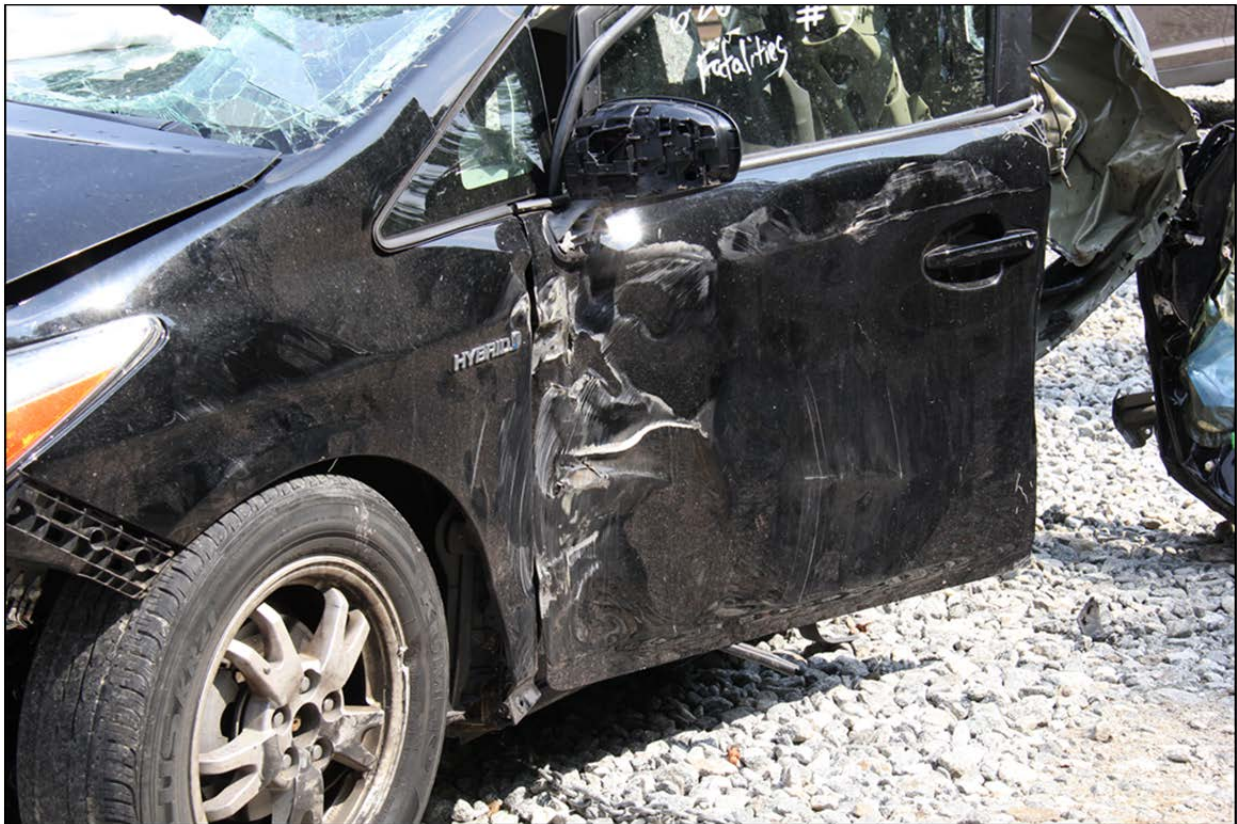
Figure 4: Photograph depicting arced scrapes and associated indentation contact damage to the driver's door on the Toyota Prius.
