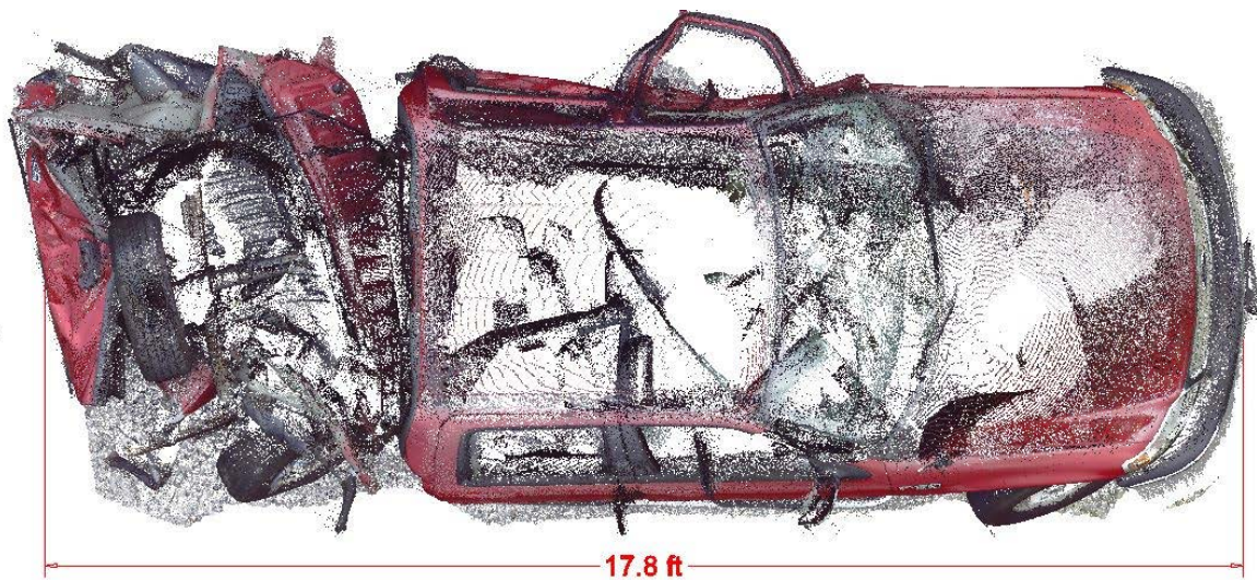
Figure 18: Overhead point cloud image of the Ford F-150 depicting certain dimensions.
