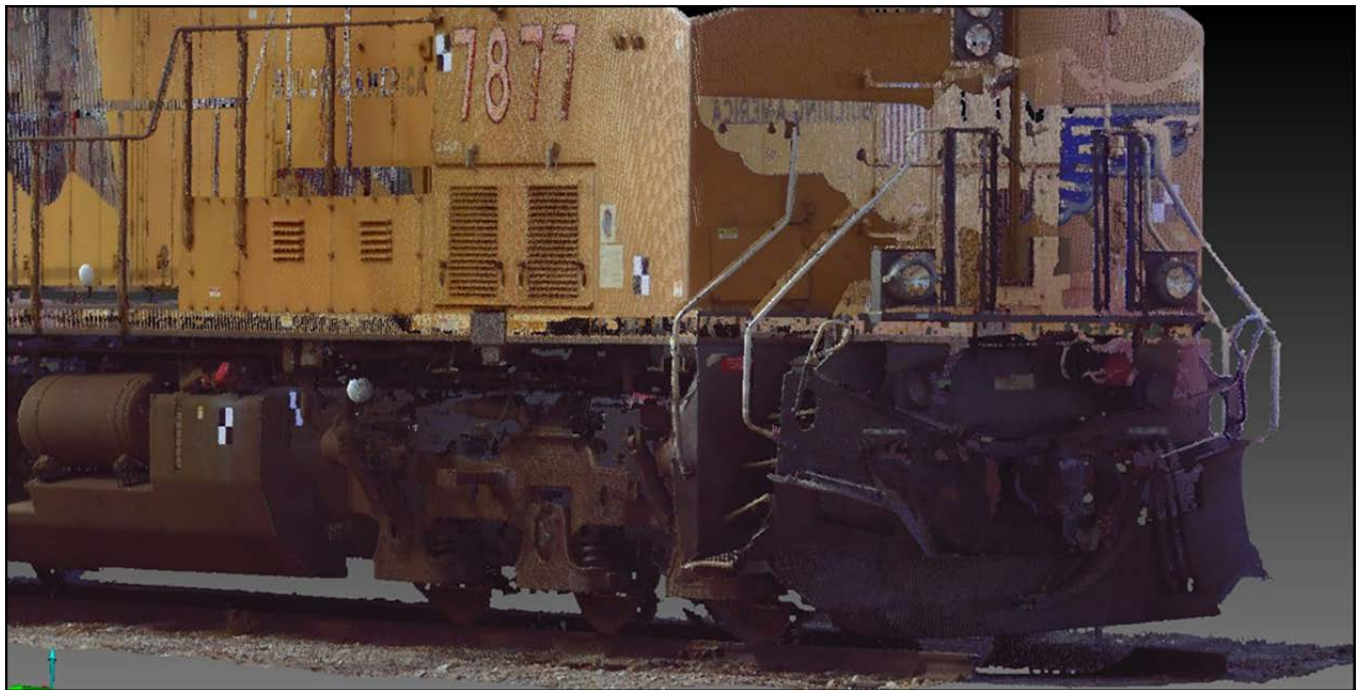
Figure 3: Depiction of linked 3D scans with focus on frontal impact area.
