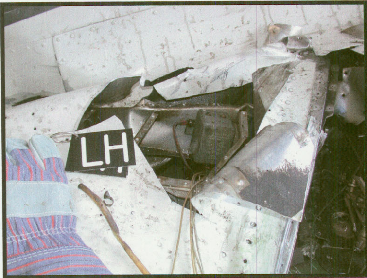
BAUK-216 Left boost pump relay
