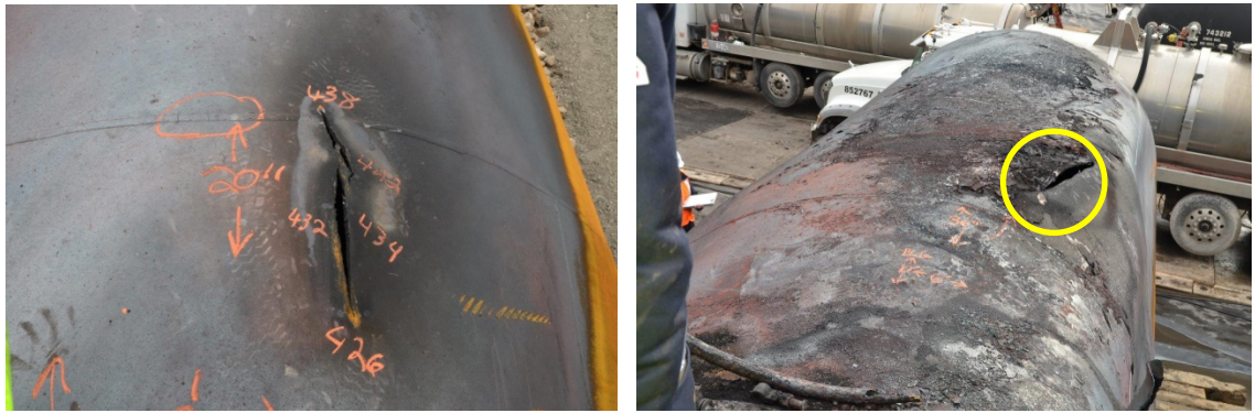
Figure 6: Examples of small thermal tears CBTX 741944 (left) and CBTX 742035 (right).
