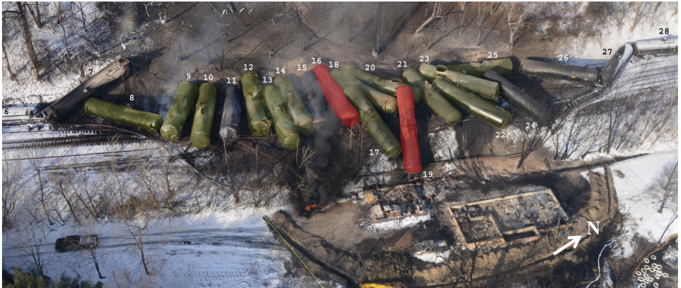
Figure 3: Tank car locations. Punctured cars are highlighted in red, cars with thermal tears are highlighted in green. (Courtesy Federal Railroad Administration, February 18, 2015)
