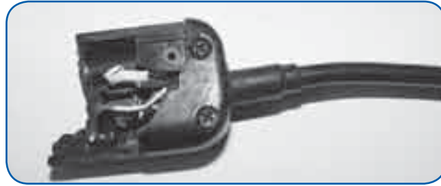
Figure 1. Fractured cord end fitting
