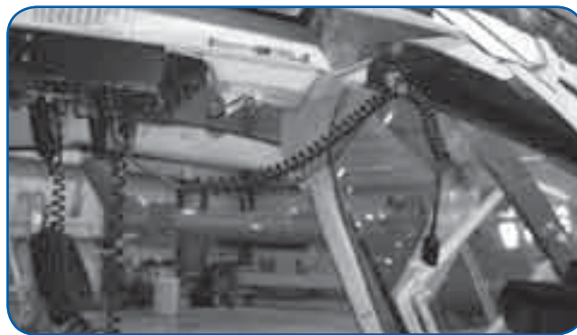
Figure 2. Intermediate helmet “pig tail” connection cords
