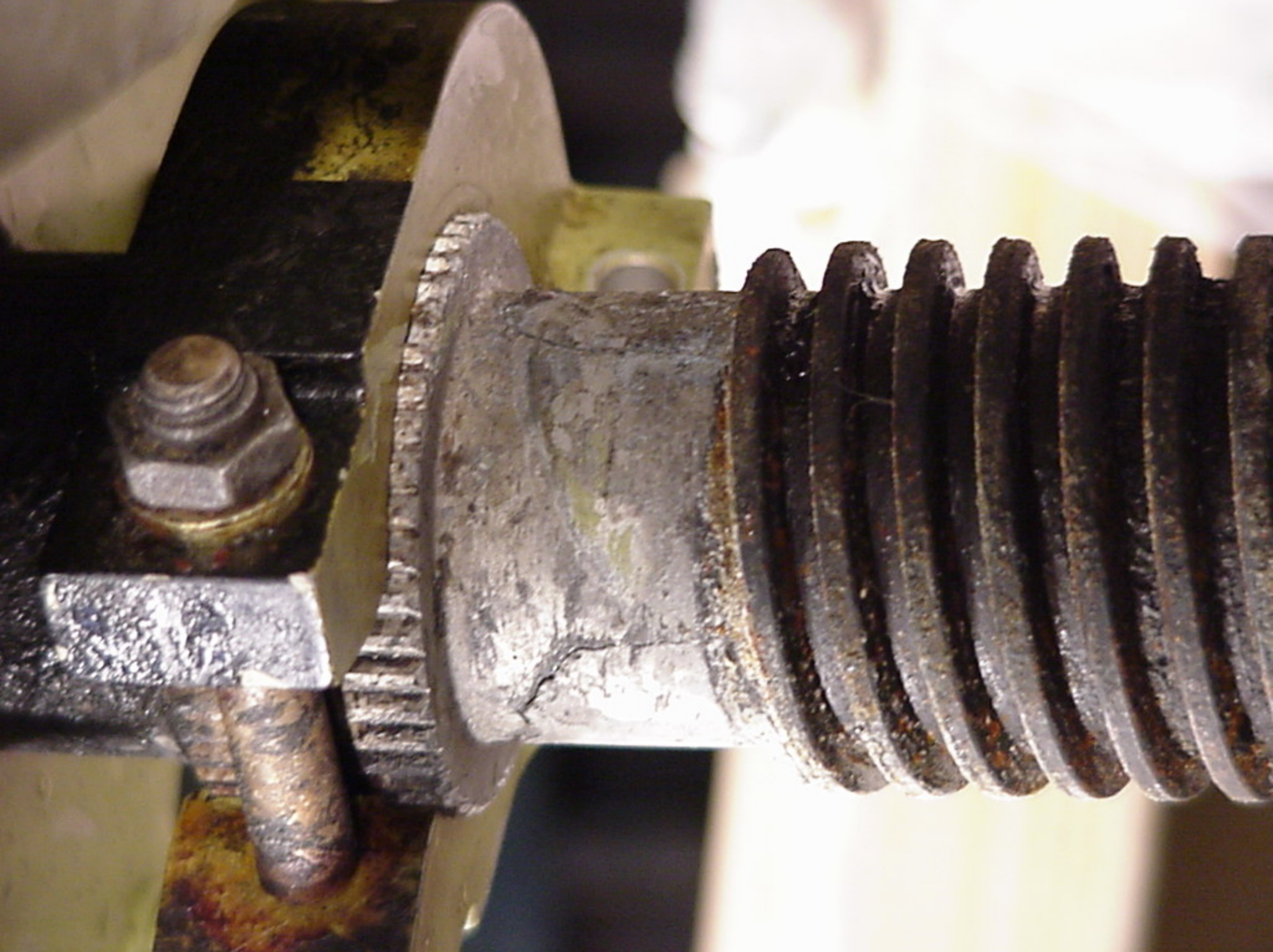
Systems Photo - Upper Stop Fracture3
