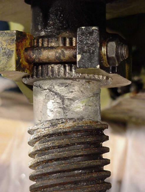
Systems Photo - Upper Stop Fracture1
