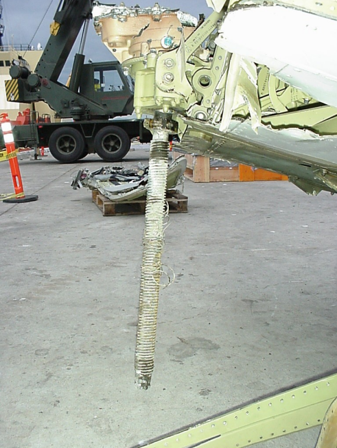
Systems Photo - Jackscrew
