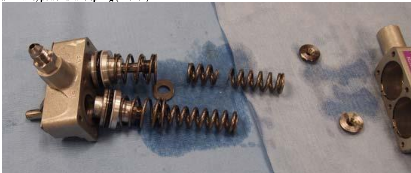
#2 Brake, power brake spring (Broken)
