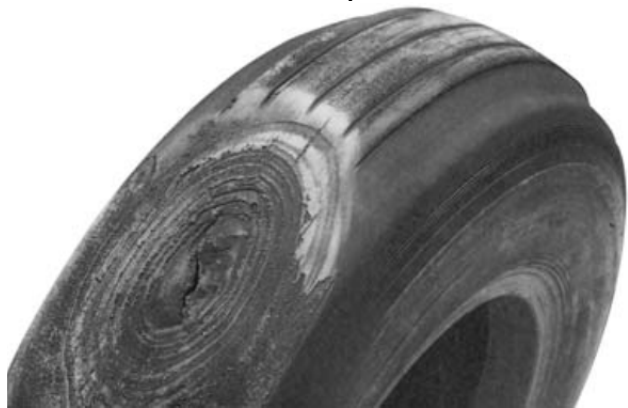
Figure 10. Photo of flat spot through tread of tire in Dunlop Care & Maintenance Manual. Caption states “Dry Braking Flats. Locked (or almost locked) wheels during a landing on a dry runway can cause a dry braking flat spot on a tyre. This is a flat scuffed surface on a part of the tread circumference.”
