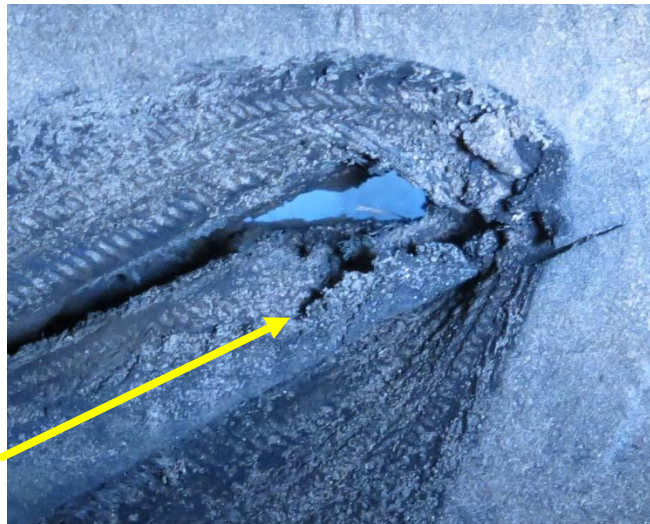
Figure 19. Detail of damage at tip of tongue in Figure 7. Note inward tear of flap at tip of arrow on tongue.
