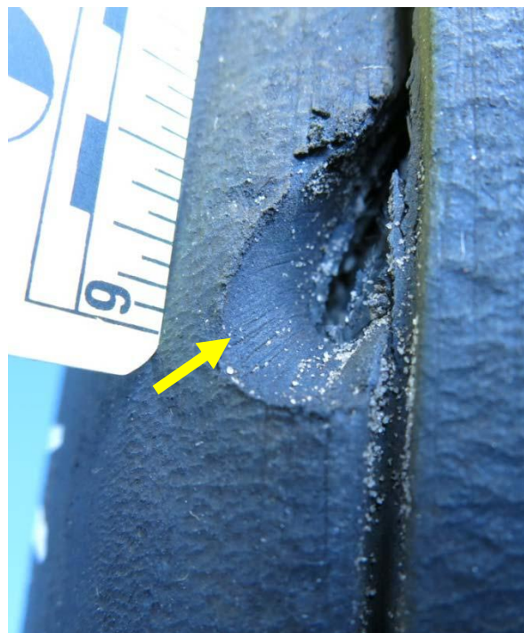
Figure 17. Detail of hole, showing striations. (arrow)
