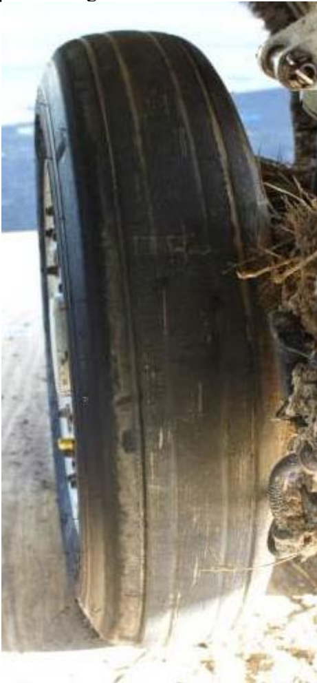
Figure 20. The tread of the #2 main landing gear tire. (Image brightness increased for visibility)
