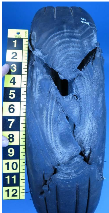
Figure 15. Direct photo of flat spot centered on tread. The 1 o’clock orientation is at top.
