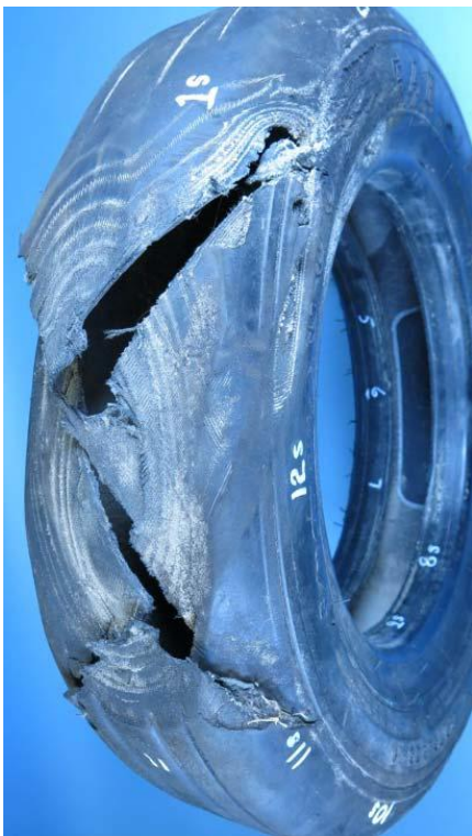
Figure 12. Oblique view of flat spot on Tire #1, showing serialized shoulder. Note numbering added for
