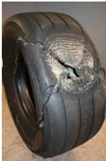
Figure 11. Michelin photograph of flat spot on tire.
