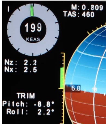
Figure 8 - PFD upper left corner of display showing airspeed, Mach, accelerations and trim indications (INS mode as noted by the “I” and gray background)
