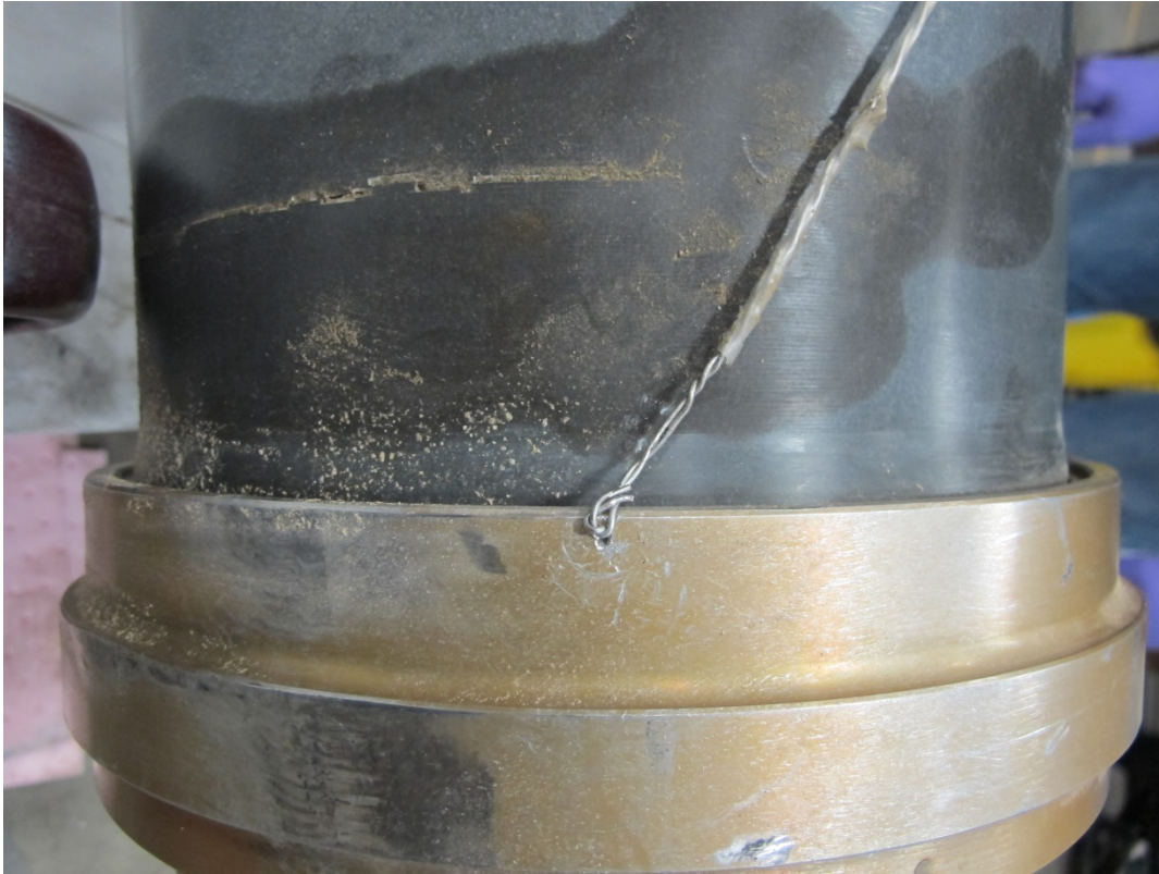
Figure 21 - The RH feather actuator breach
