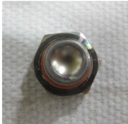
Figure 27 - Burst disc from LH regulator
