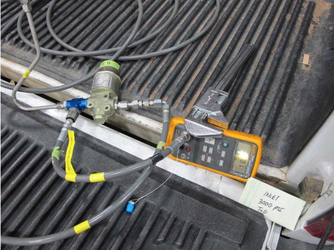
Figure A-1 – Regulator pressure test setup – Supply tank and outlet valve not shown
