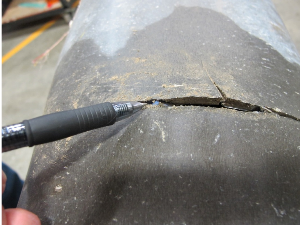
Figure 15 - LH feather actuator cylinder breach with seal exposed
