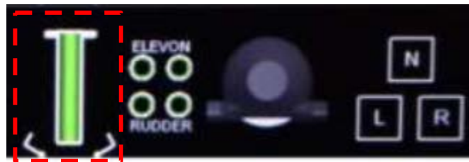
Figure 5 - Trim strip feather status display (shown unlocked and extended)
