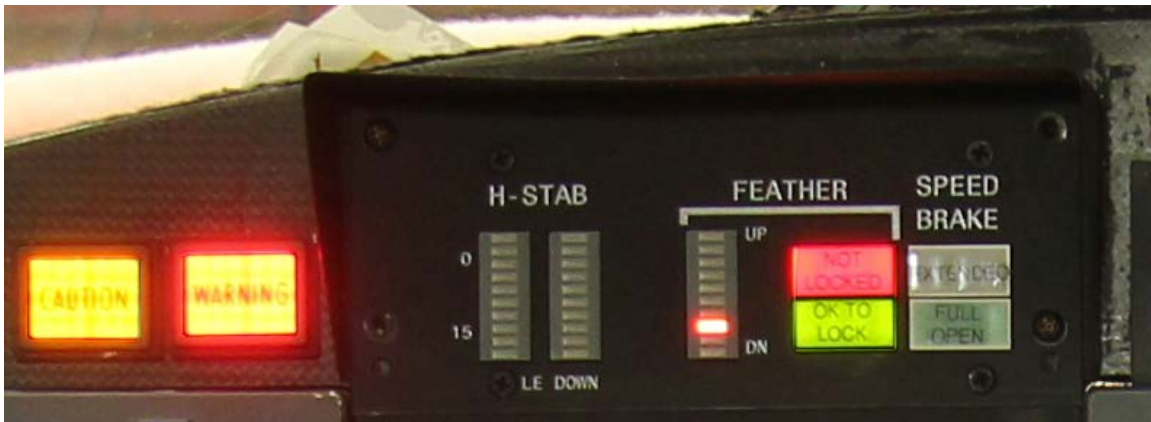
Figure 7 - Feather LED backup indicator on SS2
