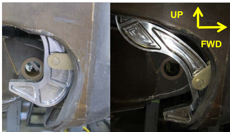
Figure 4 - Current production feather lock hook shown in the locked (left) and unlocked (right) position (note: boom and pin not shown)
