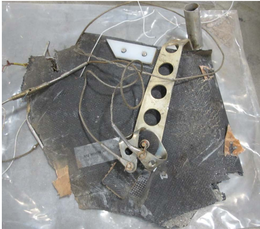
Figure 36 - LH feather unlock handle
