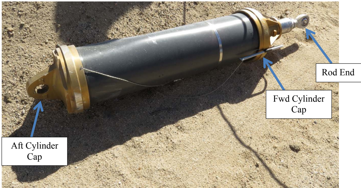
Figure 14 - LH feather actuator as found
