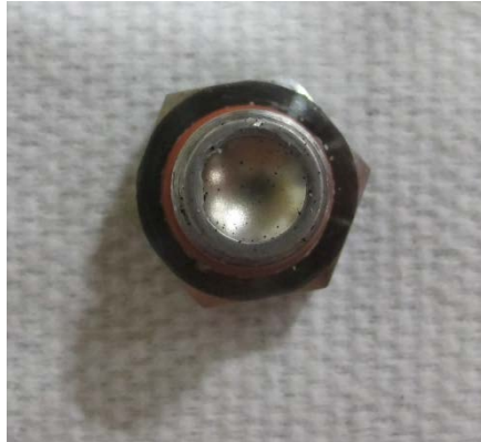
Figure 25 - Burst disc from RH regulator
