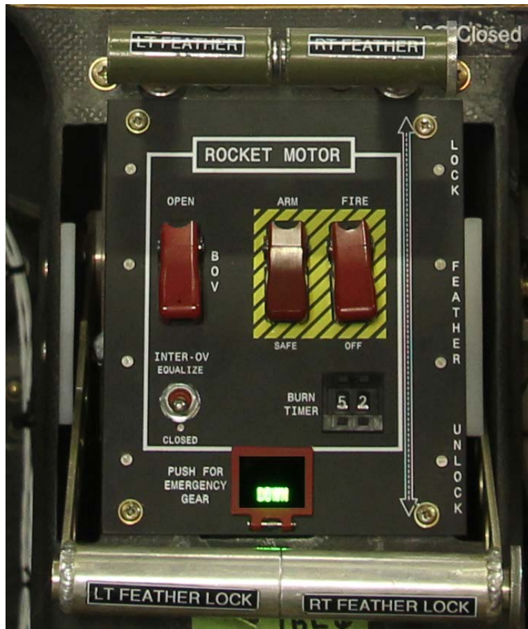
Figure 2 - SS2 feather lock and feather handles (feather lock handles shown in unlock position, feather handle in retract position) (Photo: Scaled Composites)
