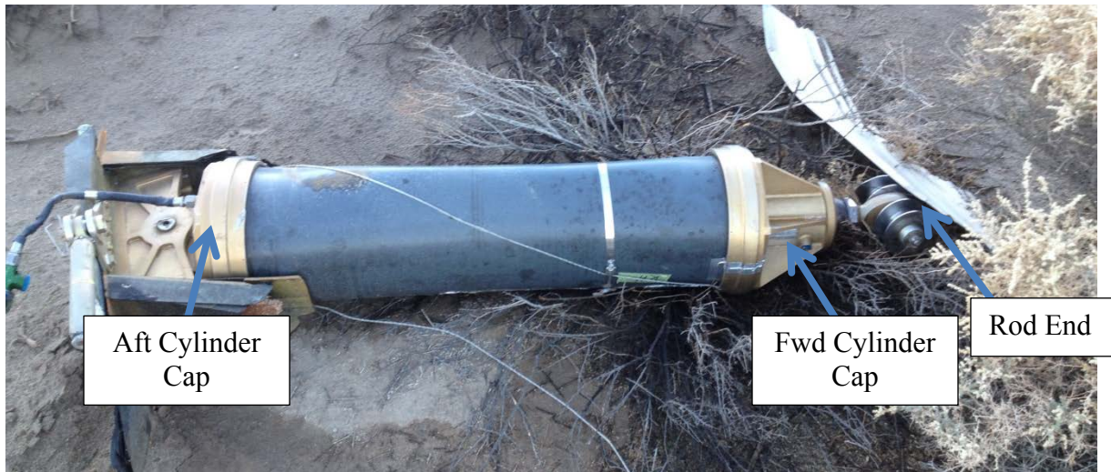
Figure 20 - The RH feather actuator as found
