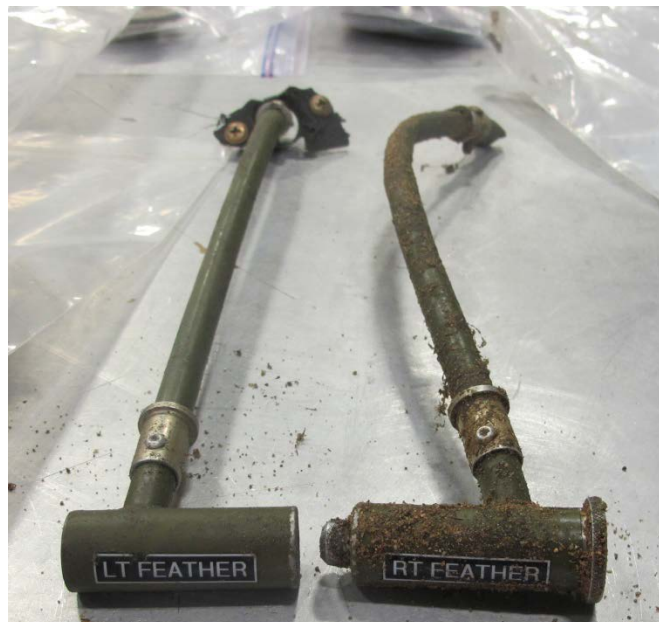
Figure 38 – Left and right feather extend handle
