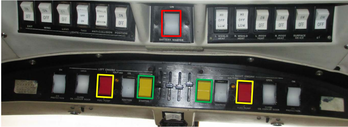
Figure 3 - Overhead panel from exemplar aircraft (older model) with, battery master, generator and fuel pump switches highlighted
