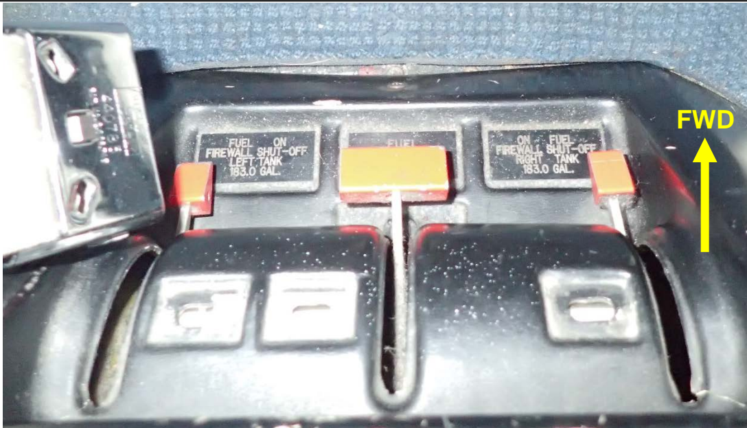
Figure 6 - Fuel shutoff and crossfeed valve panel from an exemplar aircraft (view looking down towards cockpit floor)
