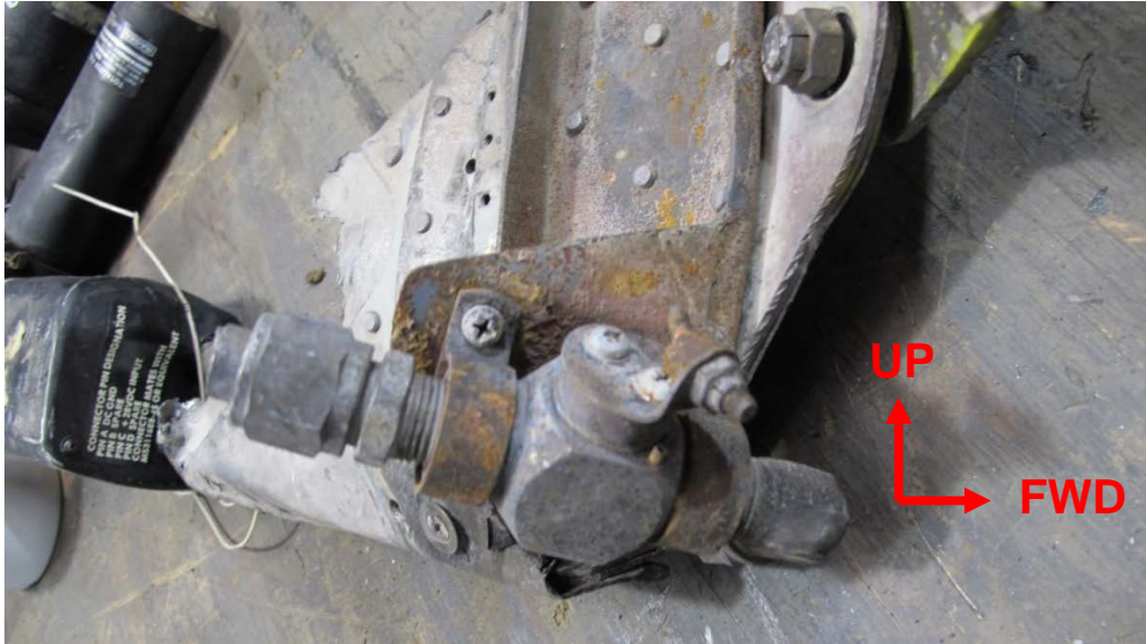
Figure 14 - Left hand Fuel SOV as recovered
