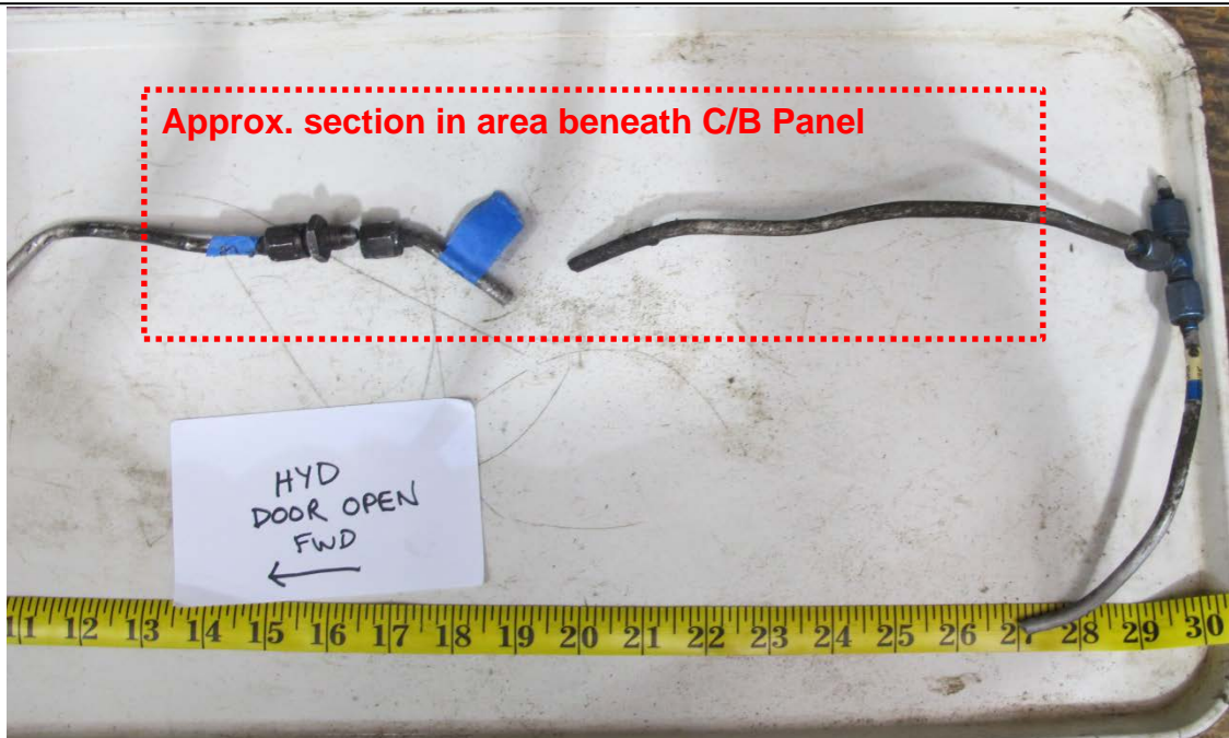
Figure 12 - Portions of hydraulic line "DOOR OPEN", with area beneath the circuit breaker panel highlighted
