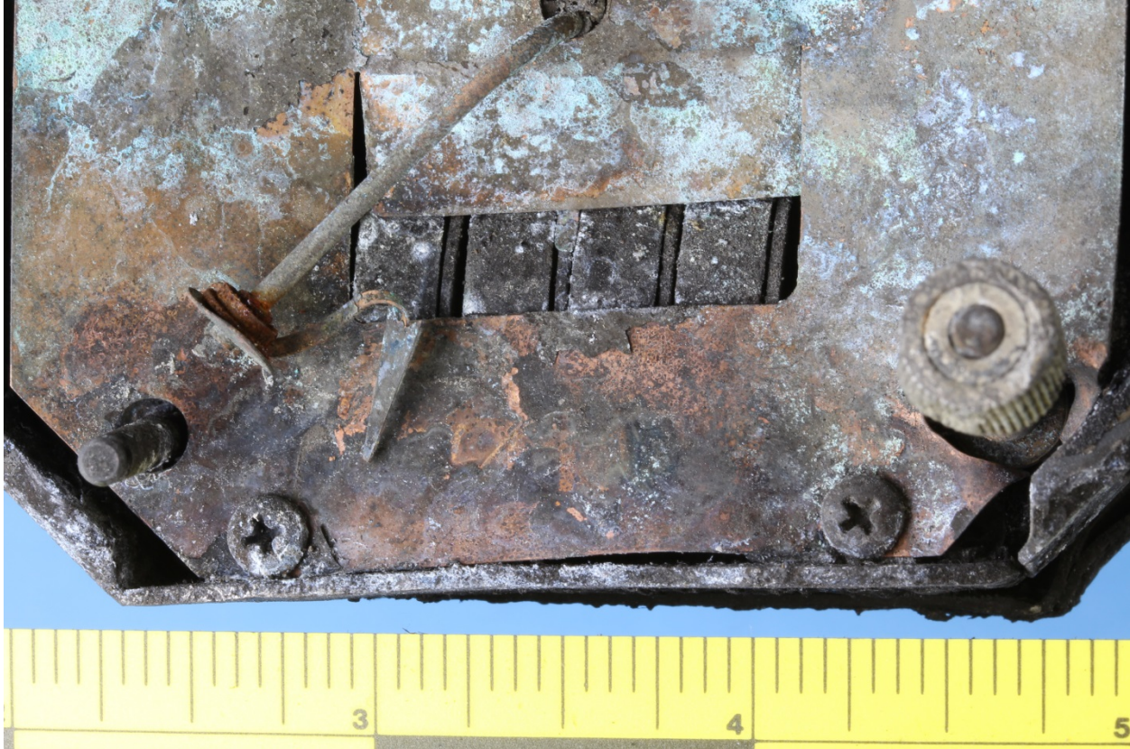
Figure 5 - Close up of Captain's Altimeter
