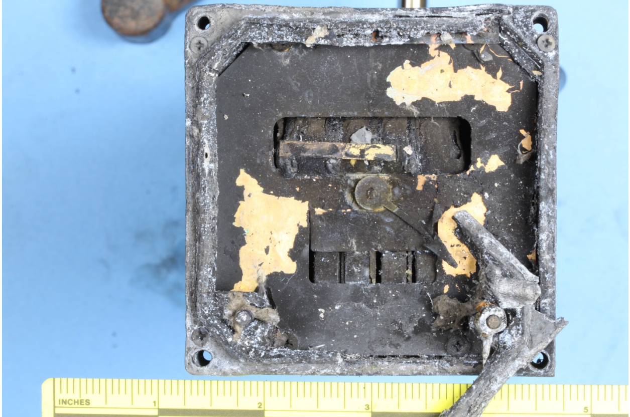
Figure 11 - Right-hand (first officer's) Altimeter
