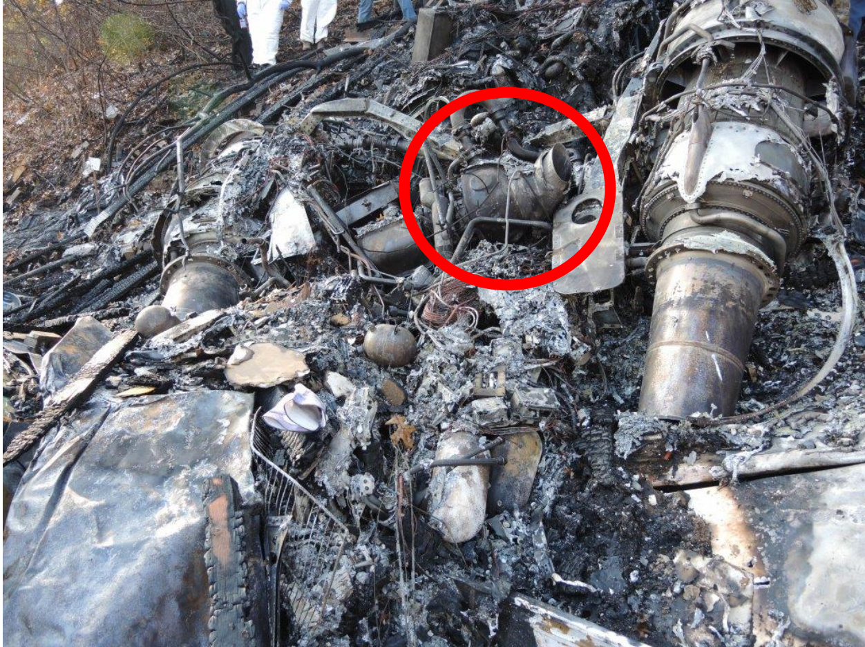
Figure 13 - Auxiliary Power Unit On-Site (Circled)
