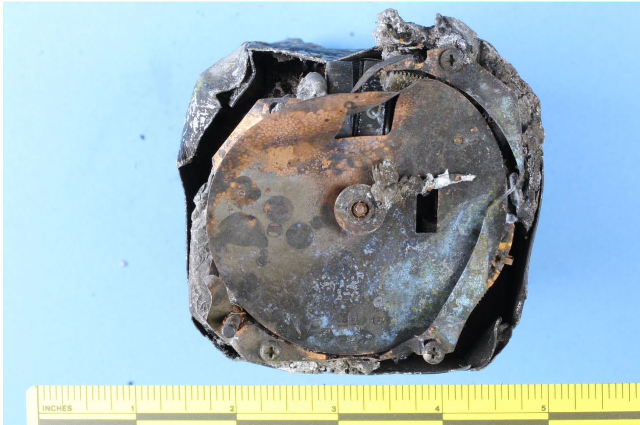
Figure 3 - Captain's (Left-Hand) Mach Speed Indicator
