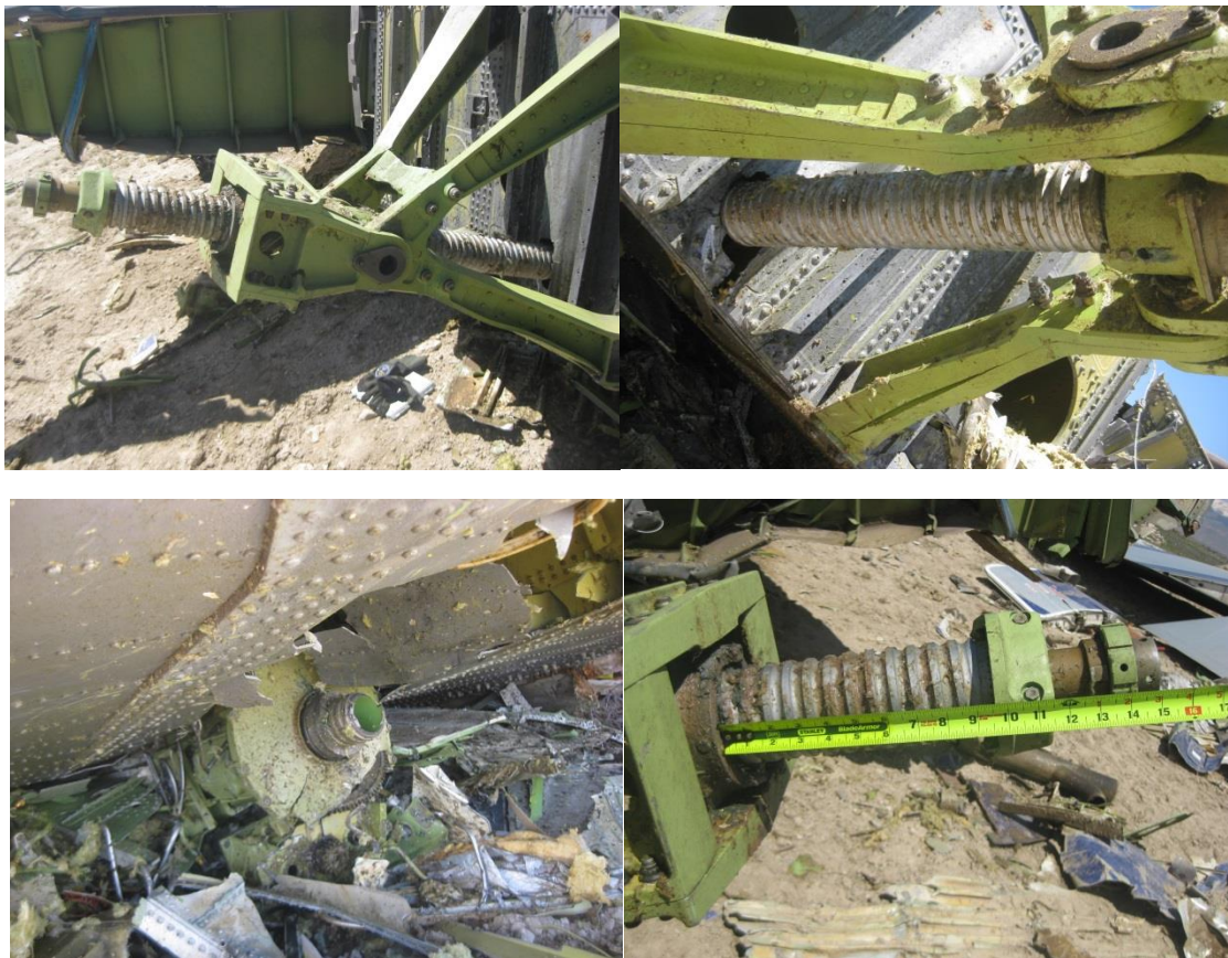
Figure 7 - Horizontal Stabilizer jackscrew segments as found
