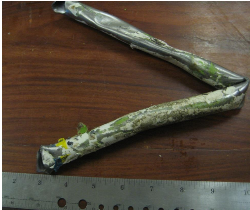
Figure 8 - Piece of hydraulic line found on Runway 03
