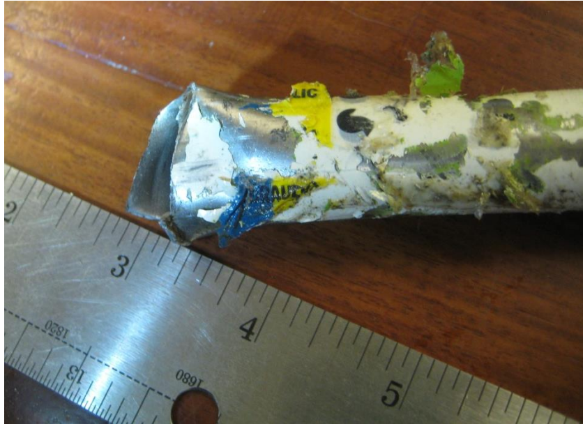
Figure 9 - Identification decal on hydraulic line
