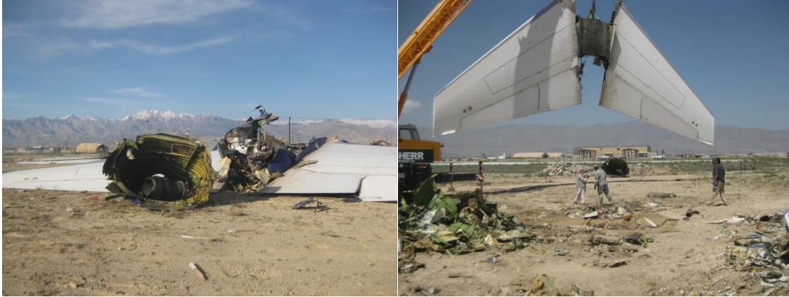
Figure 6 - Elevator and Horizontal Stabilizer segment as found (Left) and being overturned (Right)
