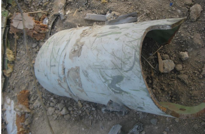
Figure 11 - Segment identified as Nose Gear Upper Cylinder
