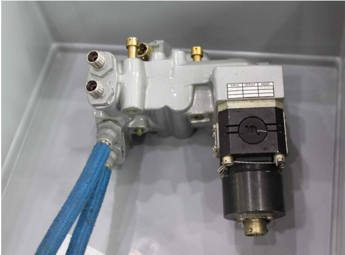
Figure 5: Steering Manifold Assembly with Servo Valve Attached
