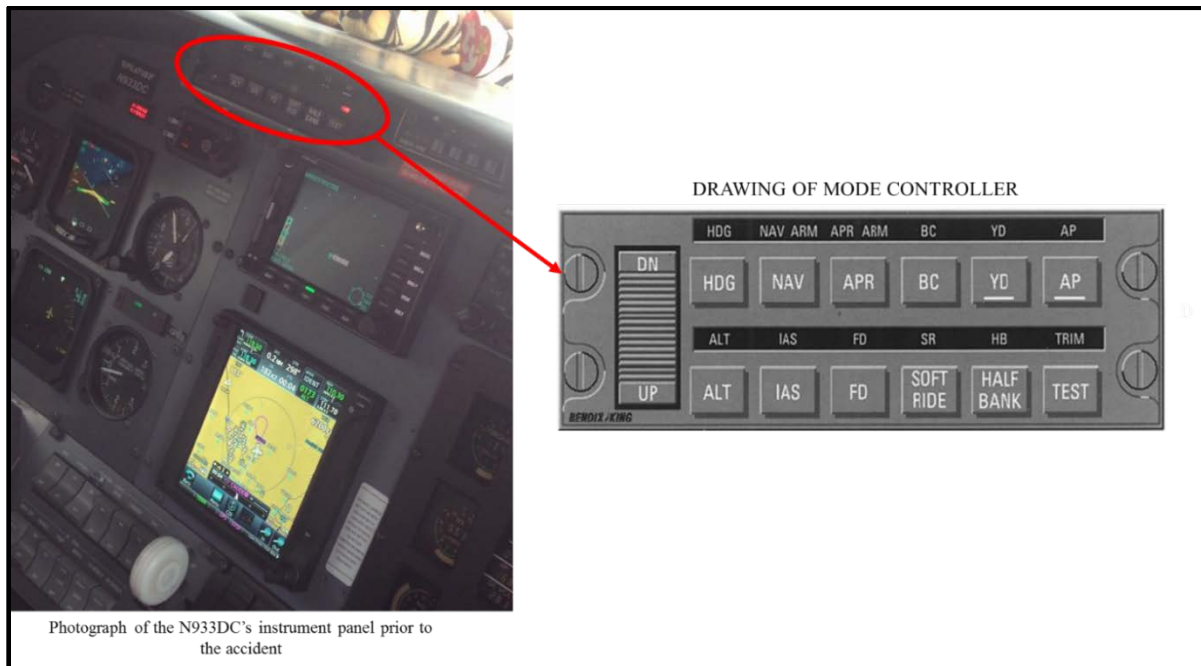
Figure 1 Location of the mode controller
