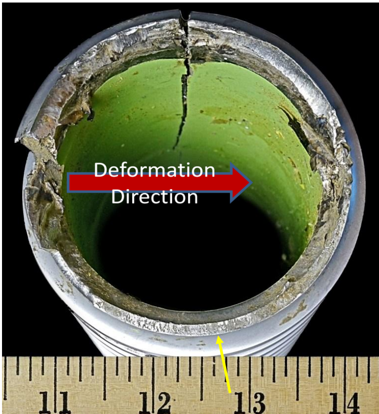
Figure 5. Optical image of the direction of the plastic deformation of the ballscrew (red arrow) relative to the origin of the fracture (yellow arrow).
