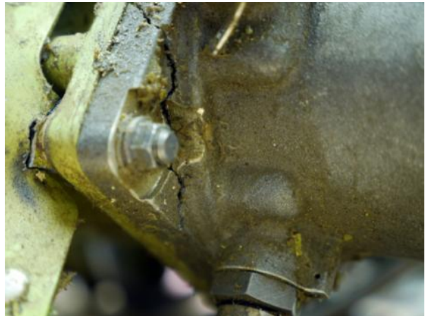
Figure 56: Right hand hydraulic motor flange crack
