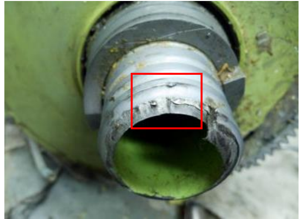
Figure 24: Witness mark near fracture surface
