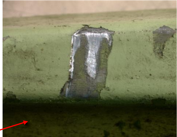
Figure 63: Forward yoke witness mark
