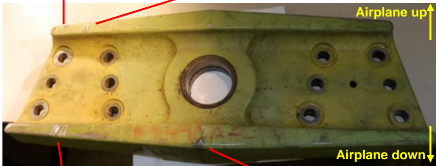
Figure 64: Upper gimble, forward yoke
