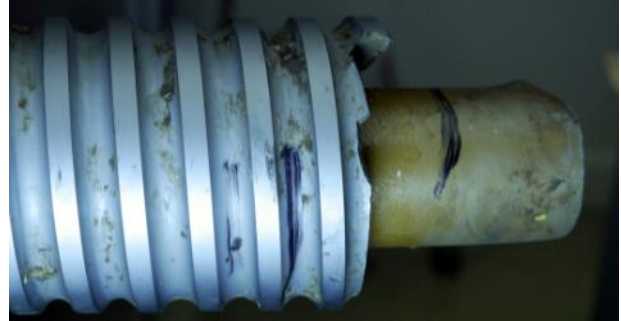
Figure 44: Witness marks on ballscrew, 180 degrees from longitudinal fracture
