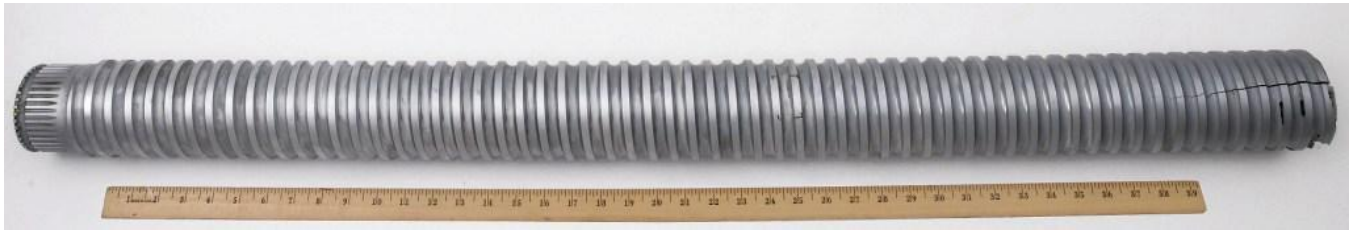
Figure 1. As received photograph of the fractured ballscrew. The fracture location is the right side of the screw and the distortion is exaggerated by the camera..
