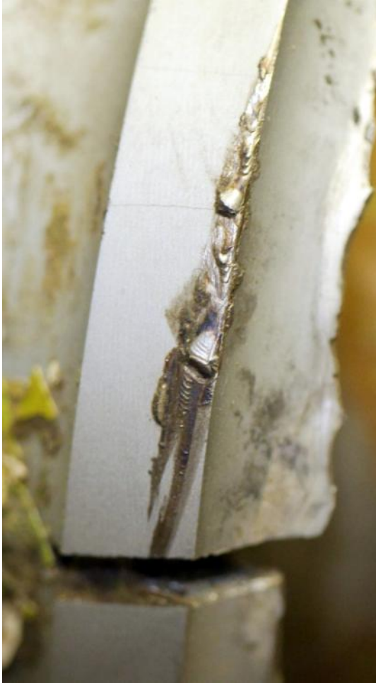
Figure 47: Witness mark on ballscrew
