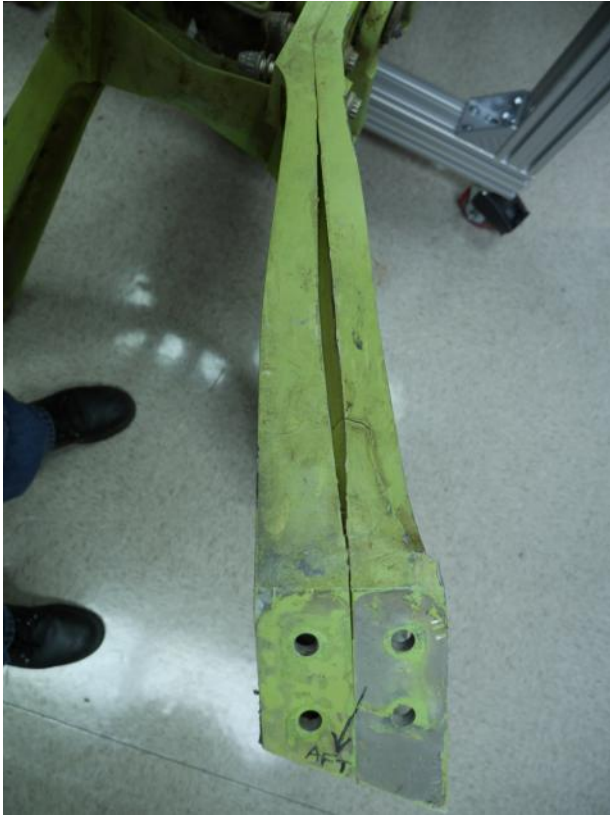
Figure 31: Upper gimble support structure, distorted and fractured leg
