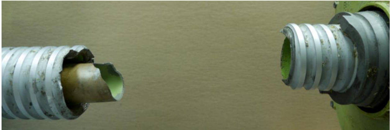
Figure 41: Ballscrew sections aligned
