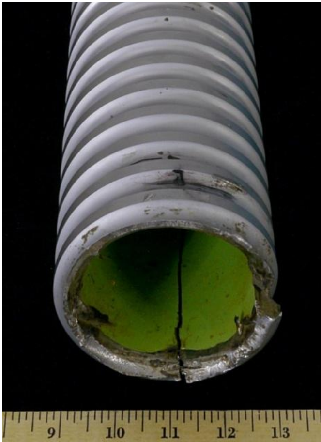
Figure 2. End on view of the fracture of the largest piece of the ballscrew.
