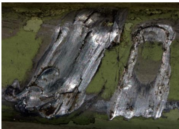
Figure 65: Forward yoke witness marks
