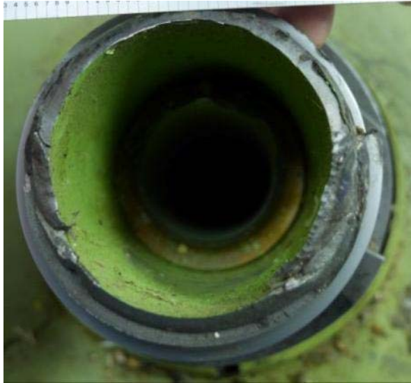
Figure 27: End view of fractured ballscrew
