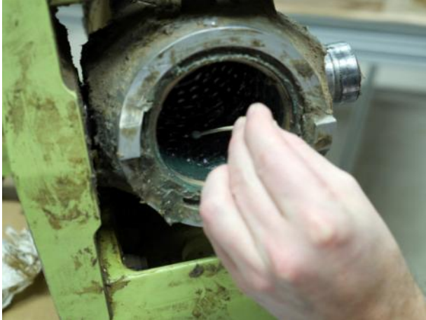
Figure 71: Grease collected from ballnut
