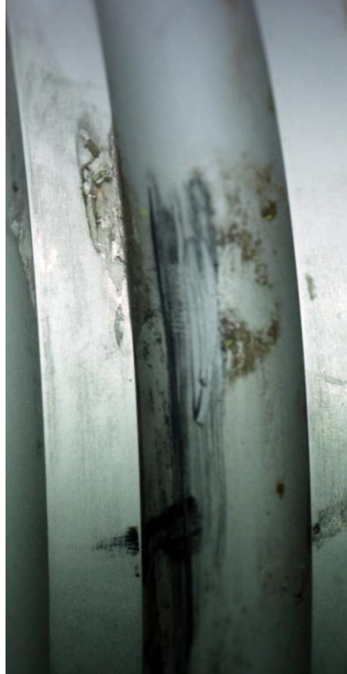
Figure 48: Witness mark on ballscrew, 180 degrees from longitudinal fracture
