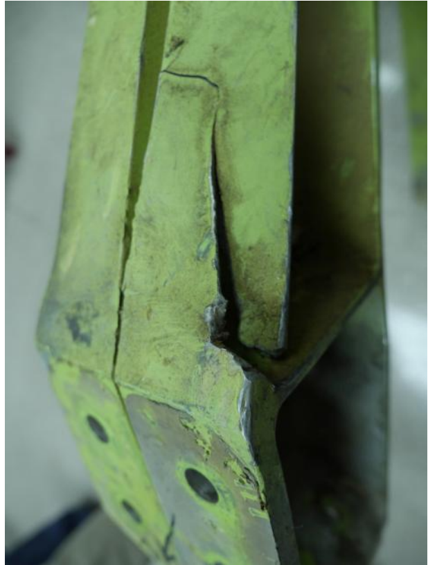
Figure 32: Upper gimble support structure, fractured leg
