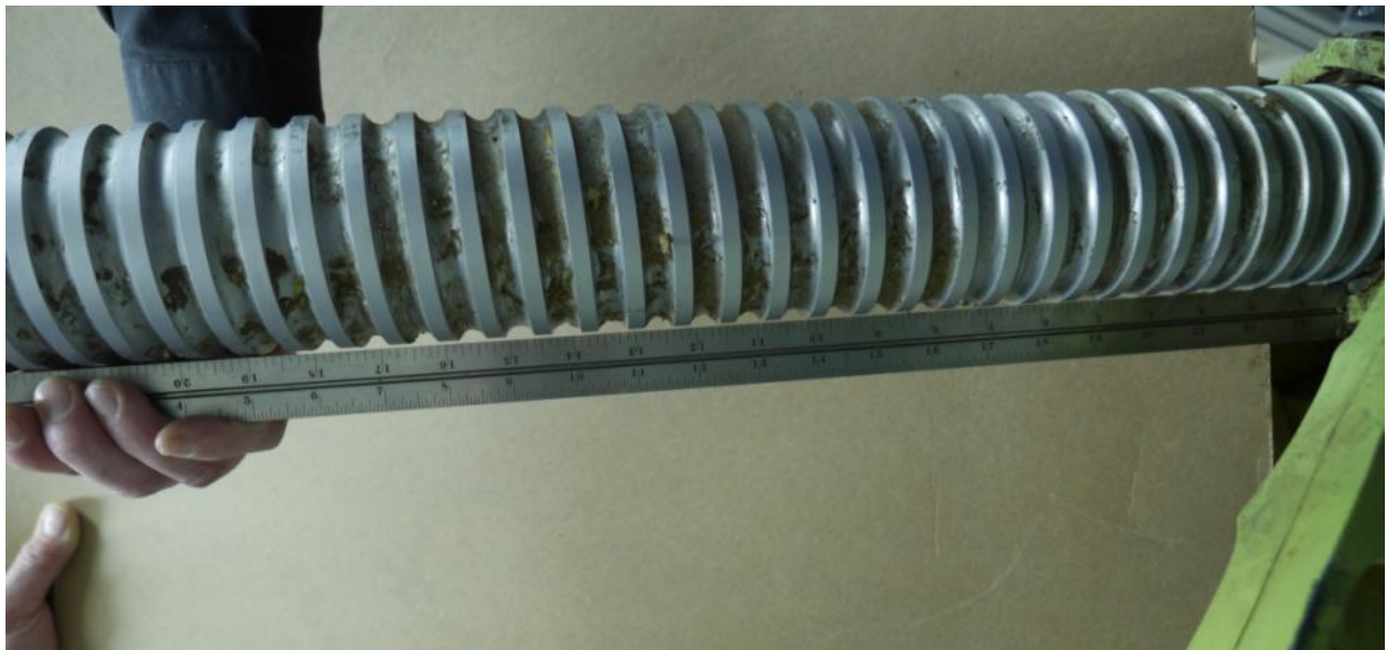
Figure 42: The ballscrew exhibited bending
