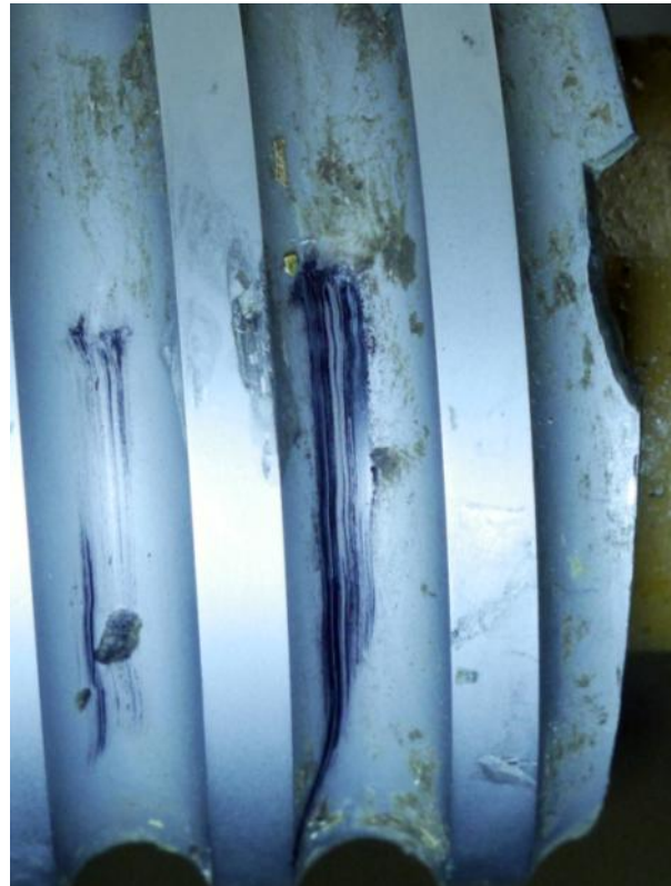
Figure 46: Witness marks on ballscrew, 180 degrees from longitudinal fracture
