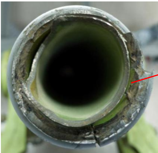
Figure 33: Fractured safety rod
