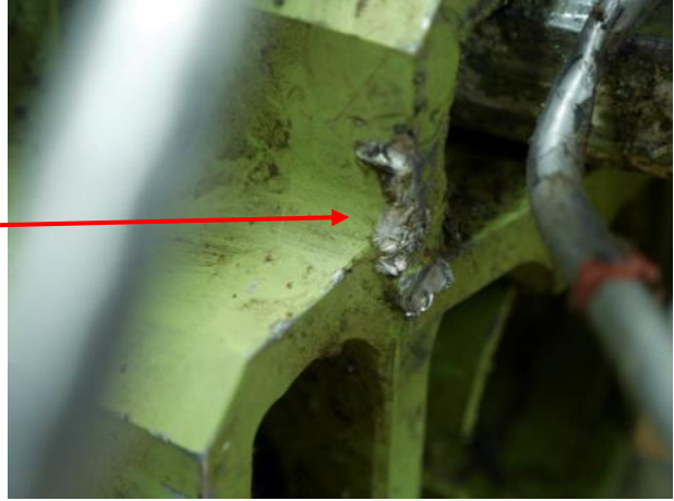
Figure 54: Lower gimble damage
