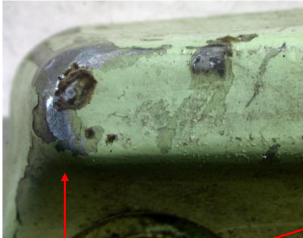
Figure 62: Forward yoke witness marks
