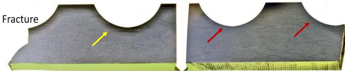
Figure 8. Metallurgical cross sections of several threads near and including the fracture. A case hardened region is shown with the yellow arrow and regions that are not case hardened are indicated with red arrows.
