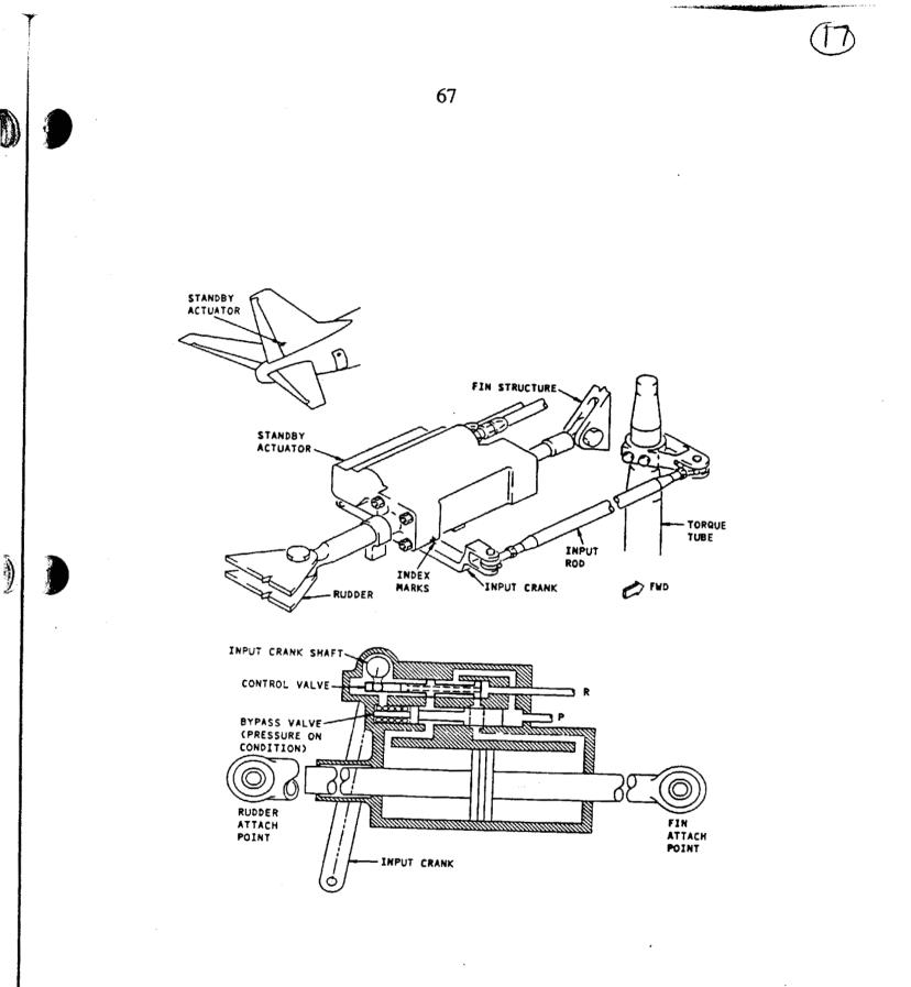
Figure 5.--Standby rudder actuator.
