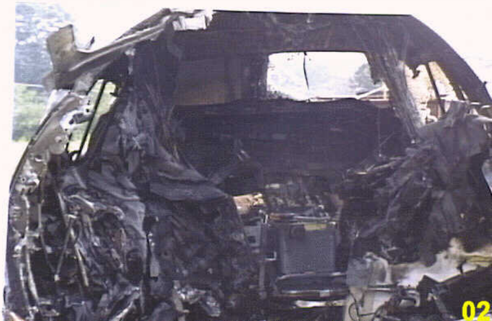
Systems 9A - Photo 02. View from Cabin looking forward toward the cockpit
