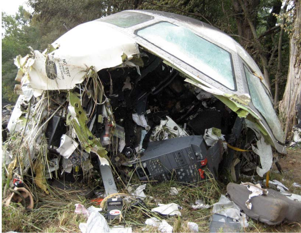
Figure 2 - Damage to Flight Deck
