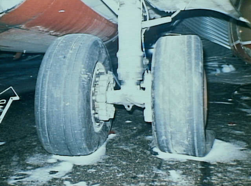
Systems 9 - Photo 6. View looking forward of the right main landing gear. Note the left inboard tire is still pressurized. (Photo by FAA)
