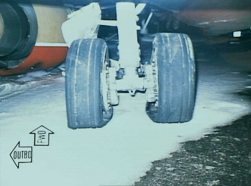
Systems 9 - Photo 5. View looking forward of the left main landing gear. Note condition of both tires. (Photo by FAA)
