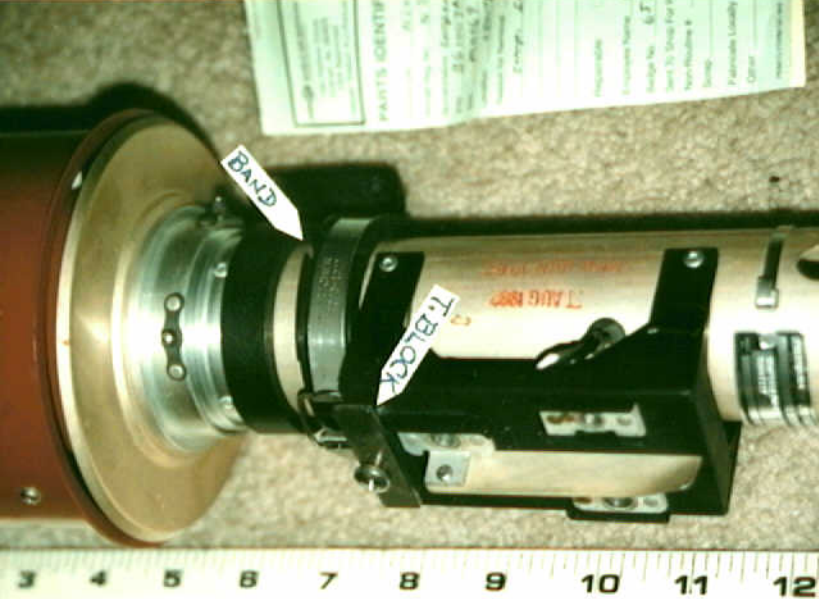
Systems 9 - Photo 48. Airplane 21. B-757 compensator with arrows pointing to where impressions were found in wiring. (Top of compensator is near "12")
