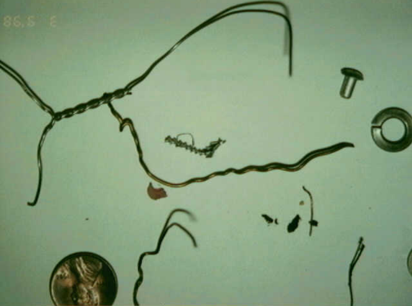
Systems 9 - Photo 45. Airplane 19. B-767 debris found immediately beneath burned area.
