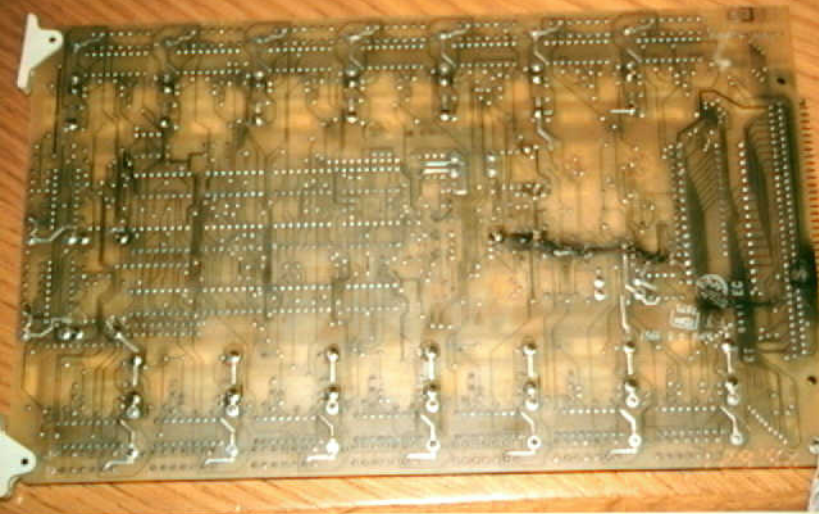
Systems 9 - Photo 44. Airplane 19. B-767 thrust reverser indication printed circuit card with burned track. Burned track was connected to the burned wire bundle through other wiring.
