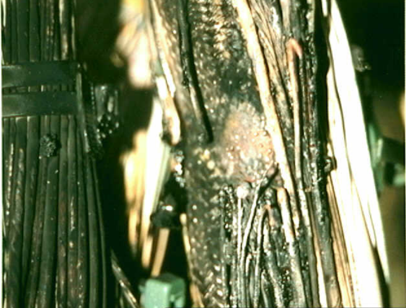
Systems 9 - Photo 42. Airplane 19. B767 detail of burned area of vertical wire bundles. The adjacent burned bundle (to left) had molten holes in wire insulation and was more than an inch away. Wire types were Aromatic Polyimide and XL-ETFE.
