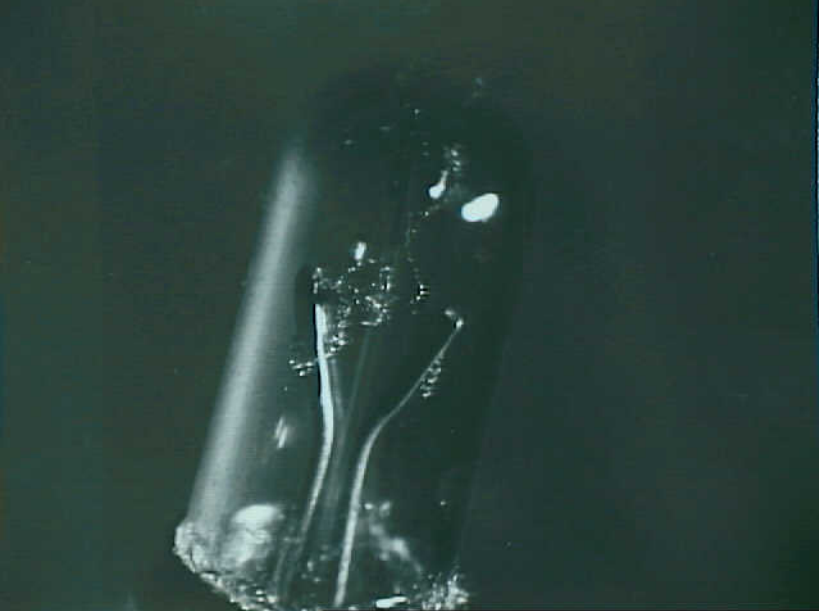
Systems 9 - Photo 4. Filament from Propeller Anti-ice "Normal" Light Bulb
