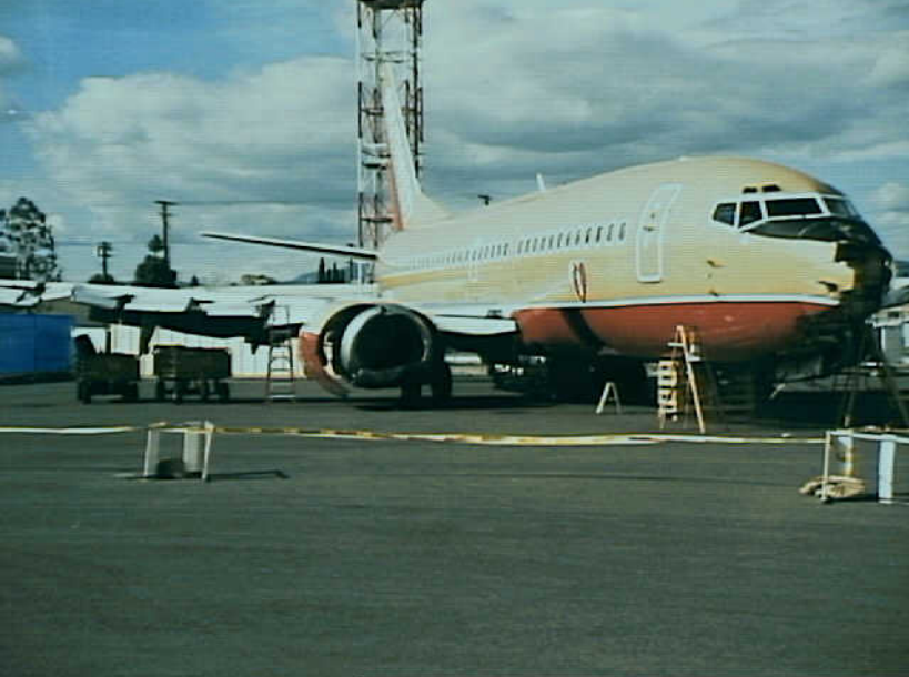
Systems 9 - Photo 3. View of N668SW after being moved. Note the damage to the nose area and forward
