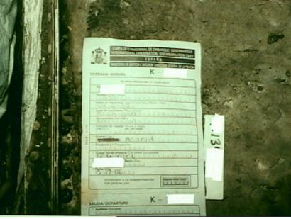
Systems 9 - Photo 28. Airplane 13. Spanish Customs form found between generator cables in 747 and laid on insulation near STA 400. Around the form are metal shavings, loose hardware, rivet fragments, and dirt. Form is dated 5-17-96.
