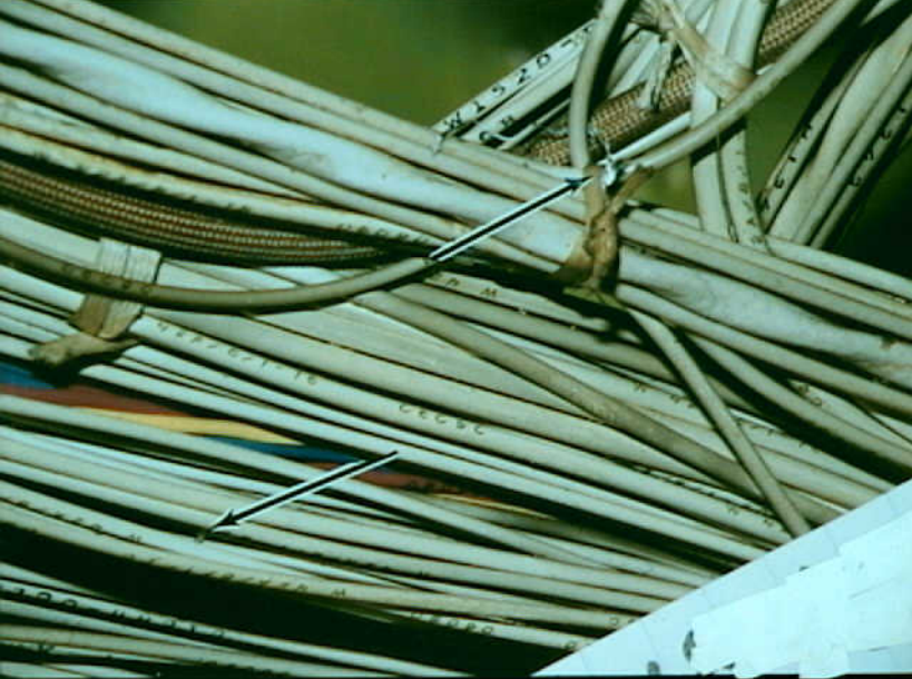
Systems 9 - Photo 22. Airplane 11. B-747 wires forward of wing spar in left raceway. Arrows point to metal shavings on wire and coming through the bottom of the bundle. Deep hot stamp letters in wire insulation at lower left have ridged edges.
