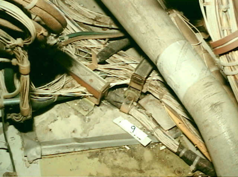
Systems 9 - Photo 16. Airplane 9. B-747 Cockpit floor behind flight engineer panel. On and between wires are dirt, lint, and metal shavings. Mixed wire types visible. (View down & forward from near right escape door)
