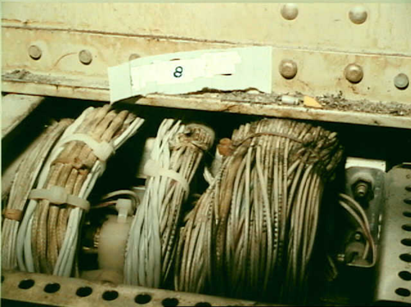
Systems 9 - Photo 14. Airplane 8. DC-9-30 in electrical equipment center at top of left power distribution panel. Visible are drill shavings and rivet fragments. Mixture of wire types is visible. Location is covered by floor boards.
