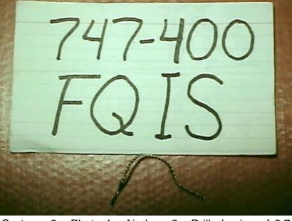
Systems 9 - Photo 1. Airplane 3. Drill shaving of 2.7 inch length, next to 3x5 inch card. Shaving found on right wing FQIS wires at wing/fuselage pressure seal in B-747-400.
