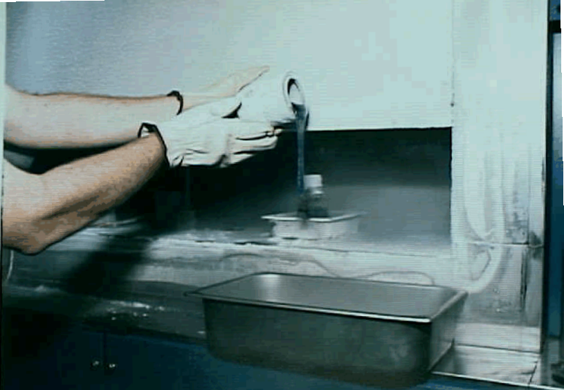
Phase 2, Photo 5. New hydraulic fluid at -110°F
