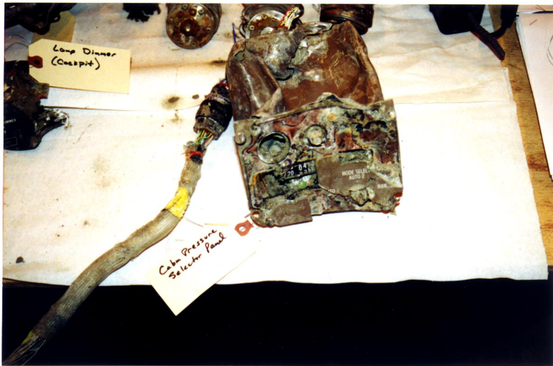
Figure 13 – Cabin Pressure Selector Panel
