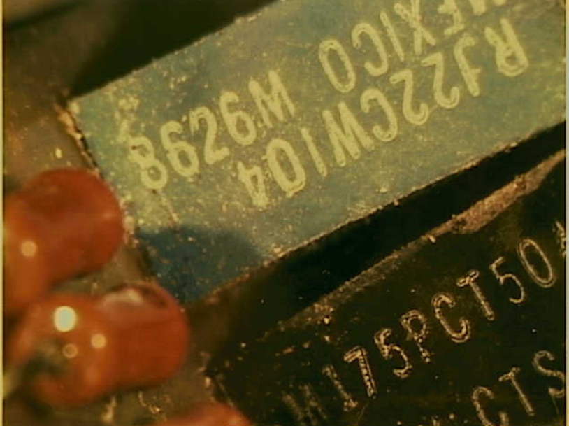
Systems 9 - Fuel Quantity Indicators - Photo 7. Totalizer component date code 8626M is visible.
