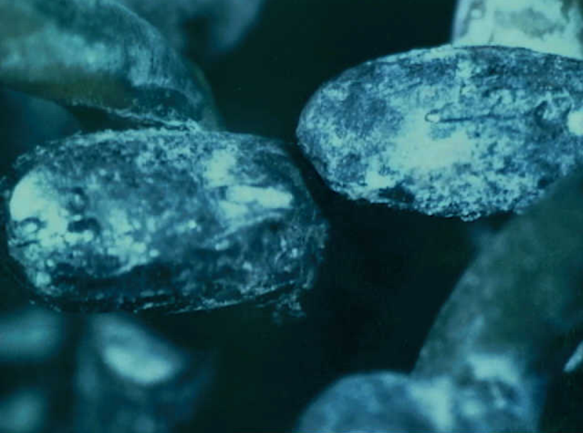
Systems 9 - Fuel Quantity Indicators - Photo 5. Totalizer (pins 3 and 11) after controlled power applications bridged the crack 3 times.
