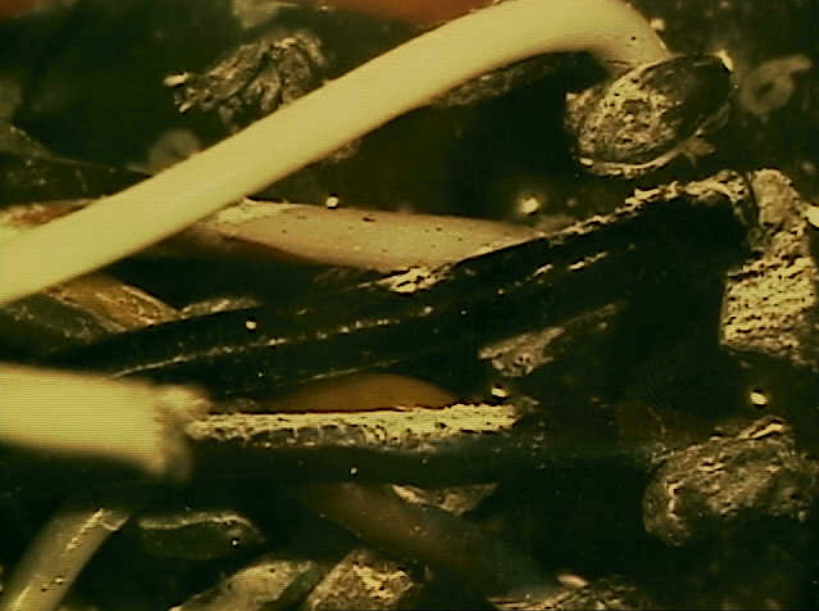
Systems 9 - Fuel Quantity Indicators - Photo 3. Totalizer connector (interior) where wires attach to pins.
