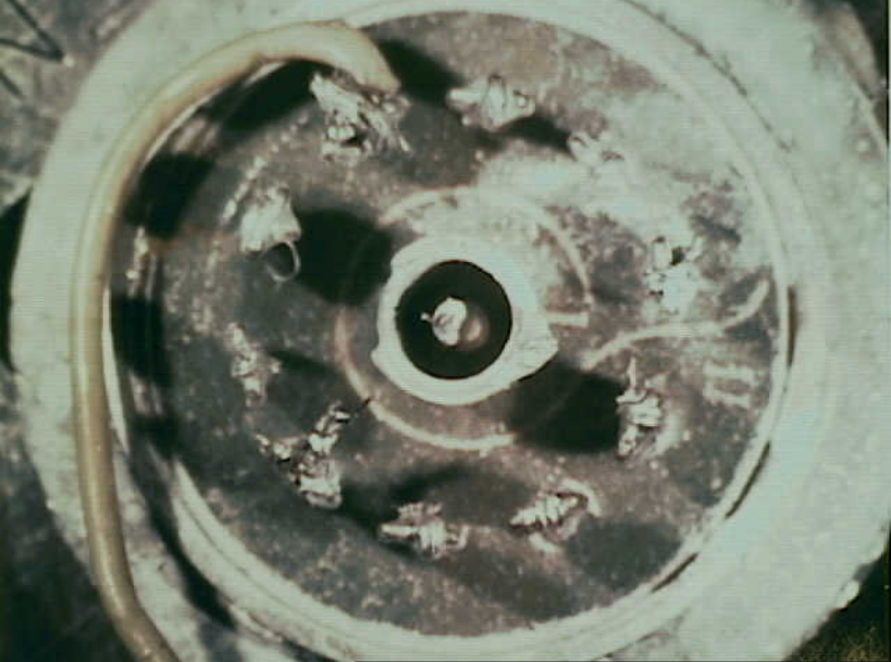
Systems 9 - Fuel Quantity Indicators - Photo 16. CWT indicator connector interior surface, as found on January 11, 1999.
